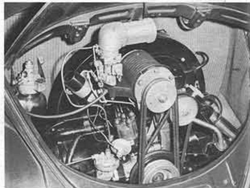
6. Install original fuel lines, connect oil line to supercharger, mount air cleaner. Installation is complete.
