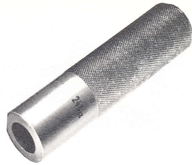
Front wheel inner bearing driver
