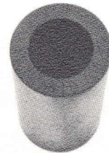
Tube for removing starter shaft bush in end plate, removing sedan king pin, and installing torsion arm link pin bush
