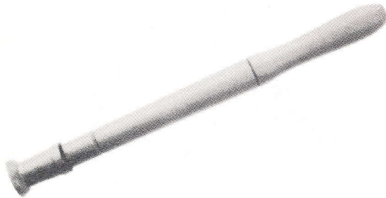
Valve lapper, 20mm rubber cup
