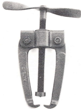
Generator bearing puller
