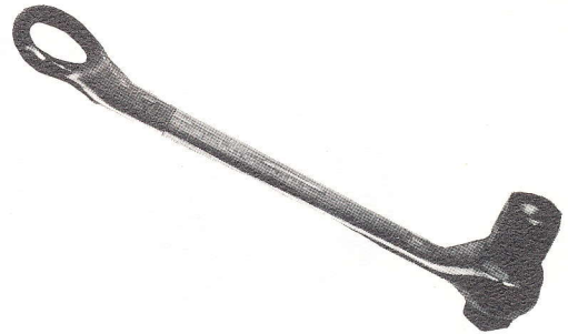
Drain plug and fan pulley wrench
