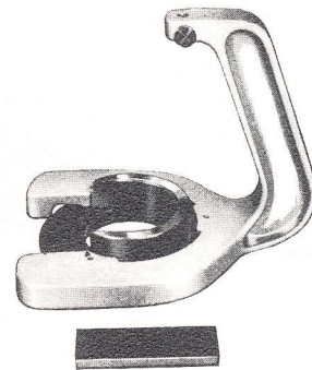
Differential housing length gage, 40hp
