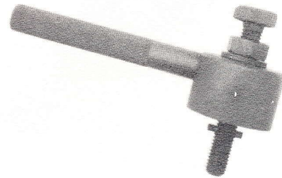
Rear axle shaft bearing installer
