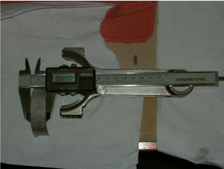
Caliper measurement of rod bearing width is compared to ground surface on crank. Note it's pretty much the same so the bearings will need to be modified and rechecked.
