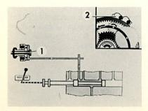
For example, when the transmission lever is in the "D" drive, position, the manual valve sends main pressure directly to #1, the forward clutch which drives the large sun gear of the planetary gear set. The ring gear of the planetary is held in position by its one-way clutch #2 and the vehicle is in first speed.
