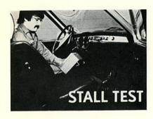
The stall speed test, checks the condition of the one way clutch in the torque converter. There are definite safety precautions that must be observed when performing a stall test:
