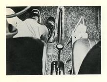
Again, with both brakes applied select Drive, momentarily accelerate to full throttle and read the pressure, then select Reverse and do the same.
