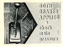
From inside the vehicle, with both brakes applied, select Reverse and check the main pressure.
