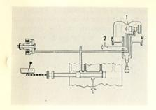
Main pressure (shown in red) is also available to the governor #1. The governor is a centrifugal valve attached to the transmission pinion shaft.
