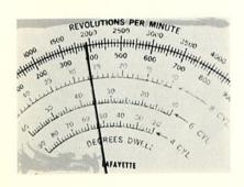
Then, start the engine and select Drive. Fully open the throttle and read the highest RPM.
