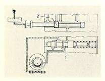
From the main pressure valve #1 main pressure goes directly to the manual valve, #2 which is directly connected to the shift lever and directs pressure to other parts of the valve body.
