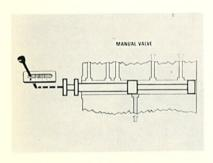
An incorrectly adjusted manual valve can cause clutches to drag and wear, by allowing main pressure to leak in and partially apply them.
