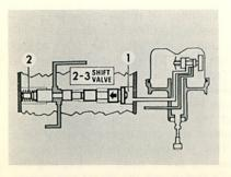
Looking at a diagram of the shift valves and governor in third gear will help us understand how we can down-shift automatically. Governor pressure #1, is the only force opposing that of the 2-3 shift spring #2. In order to move this valve to the right and shift to 2nd, we must either lower governor pressure #1 by slowing down, or increase the force on the 2-3 shift spring #2.
