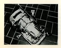
The second type of controls, the automatic controls, include pressure from the governor A, and throttle pressure from the vacuum unit B. They also work through the valve body.
