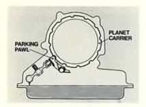
The parking pawl is a simple mechanical linkage that engages a pawl into teeth on the planet carrier, thereby locking the rear wheels. If the car is moving and the carrier is rotating rapidly, when it won't engage because the shape of its teeth will cause the pawl to be pushed out against spring tension.
