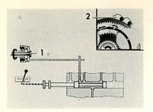
Let's review this shift sequence. When the shift lever was placed in drive, the manual valve directed pressure to the forward clutch, and the planetary's one-way clutch held the ring gear.
