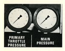
To check pressure attach the transmission gauge set to the transmission.
