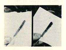
Too much ATF as well as too little can cause incorrect operation. Too much ATF may foam, allowing air bubbles into the valve body, which will disturb the hydraulic controls. While checking the level, pay particular attention to the condition of the ATF. If it is contaminated or looks or smells burned, it is an indication of mechanical problems within the transmission.
