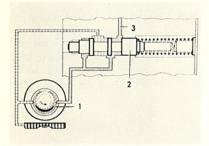
From the pump #1, pressurized ATF passes to the main pressure valve #2, which maintains a specific working pressure #3 for the hydraulically operated clutches, brakes, and transmission controls. Excess ATF is returned to the transmission sump.
