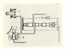
Further acceleration increased governor pressure to the point where it moved the 2-3 shift valve which allowed pressure to release the second speed brake band, and apply the direct and reverse clutch ... and so move into 3rd speed.
