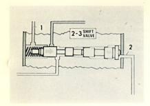
To increase the force on the 2-3 shift spring throttle pressure our second automatic control #1 is admitted to the spring end of the shift valve, overcoming governor pressure #2, causing the valve to move to the right. This shuts off pressure to the direct and reverse clutch and to the release side of the second band. The band takes hold—and the transmission shifts to second.
