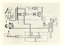
As the vehicle accelerated it increased governor pressure, this added pressure moved shift valve 1-2, which directed pressure to the second band, and the transmission shifted into 2nd gear.
