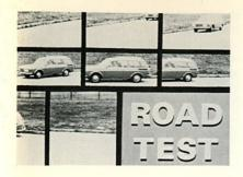
After the basic checks have been made the next step is the road test. The purpose of the road test is to see if the transmission shifts properly at the correct speed.
