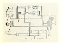
As road speed increased, governor pressure (blue) increases until it overcomes the 1-2 shift spring #1. The shift valve moves to the left, allowing main pressure (red) to go to the second gear brake band #2. The brake band is applied, and the transmission automatically shifts to second.
