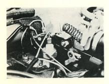
The type 3 kickdown switch is near the throttle shaft mounted on the intake air distributor.
