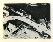
For this reason, it is critical that the cable (green arrow) be adjusted so that the manual valve #1 is fully seated. This means the parking pawl spring #2 must be compressed.
