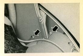
9/39 The hose is positioned at the protruding edge in front of the hinge below the moulding since water could enter the vehicle at the moulding and give a wrong impression. Use sealing compound here too if leaks are located and then touch up with paint.
