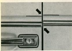
9/4 The striker plate has to be removed when commencing with door adjustments as otherwise the door fit cannot be correctly checked. The waistline shown here is very helpful. The better the door fits with the striker plate removed the less corrections will have to be made later when adjusting the striker plate. This fact also lengthens the life of the lock.
