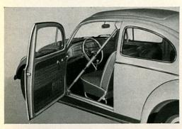
9/5 Here you see expanders being positioned in the door opening. In the case of an incorrectly fitting door, the door opening and not the door itself has altered. This alteration has been caused by the body which has settled.
