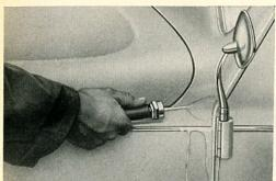
9/43 The seam at the joint between roof and front panel need only be sprayed, and sealed if necessary, on vehicles up to August 1959.
