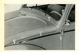
9/36 Since the leak occurred at the left side member we must try and locate it on the left side of the vehicle.
