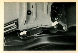
9/32 A damaged body seal often causes leaks. A seal which has been crushed by overtightening the body mounting bolts cannot fulfill its purpose. The mounting bolts may only be tightened with a torque wrench.
