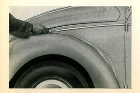
9/37 The water here is coloured to give a better illustration. A weak stream of water flows down along the beading.
