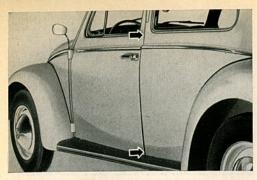
9/11 The ingress of water shown here would have been eliminated in an efficient workshop. It can be seen clearly that the door is protruding at the bottom whereas at the middle it is flush with the rear quarter panel.
