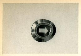
9/42 It is quite obvious that this cap must be replaced. Make sure that it is enserted into the hole prior to the installation of the moulding. Clean up the sharp edge beforehand.
