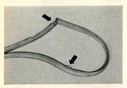
9/13 Another point. Incorrectly fitting doors usually cause damage to the door weatherstrip. It is generally necessary to replace this weatherstrip when carrying out adjustments of the door.
