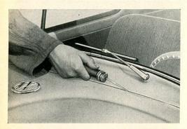
9/44 In the case of the front hood the water should be directed so that it flows along the edge of the hood in front of the windshield.
