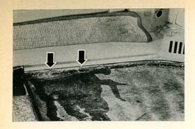
9/35 In this vehicle the water appeared at the side member after approximately half an hour. It would be useless to seal at this point as the water would run on and leak elsewhere.
