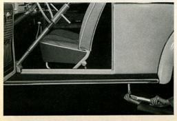
9/6 If the door fits correctly, insert the expander again in the door opening and tension it slightly. Now tighten the chassis mounting bolts to prevent the door opening from altering its shape. Use a torque wrench and tighten the bolts to 14 ft. lbs.
