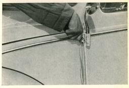
9/40 The holes for the moulding clips are provided with rubber caps. The shape of these caps was altered in August 1959 to improve their sealing efficiency.
