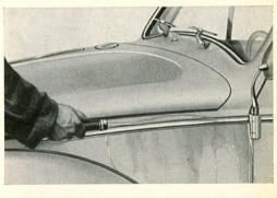
9/41 If leaks occur at the mouldings, the rubber caps are damaged. The arrow indicates a cap which has been cut by the sharp metal and now leaks.
