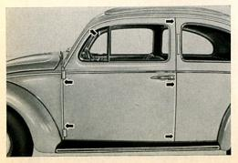
9/14 The examples just given should have the following results: The door fit is correct when the door bears evenly and the gap between door and lock pillar is .16". Only then is the striker plate installed and adjusted.
