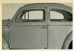
9/3 Inefficient servicing can often result in leaks and noises and it is often possible to eliminate two complaints of the same time. The first example: The arrow points towards the incorrect door gap. In the upper region the door nearly bears on the lock pillar whereas the gap shown by the lower arrow is too large.
