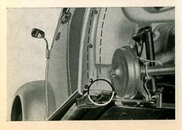
9/27 Spray the vehicle from behind the wheels. Another mechanic should use a flashlight to observe the interior.
