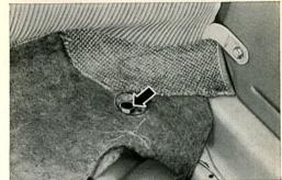
9/9 and this bolt which attaches the rear quarter panel to the chassis. Back off both bolts approximately 5 turns.
