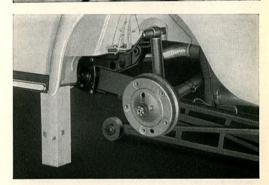
9/10 Insert a synthetic packing .16" thick made from the guide plate of the sliding roof into the gap. A metal plate is not suitable as it could cause squeaks.
