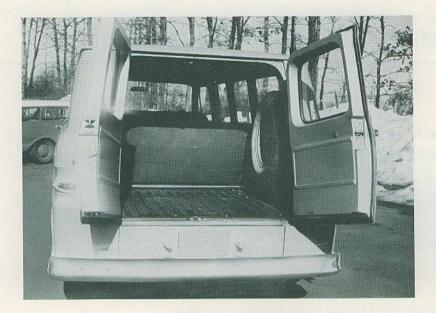
The Greenbrier, with none of these "deluxe" features, has a bare metal luggage compartment containing the spare tire and lined with the metal engine compartment lid which must be removed along with luggage to reach the engine.
