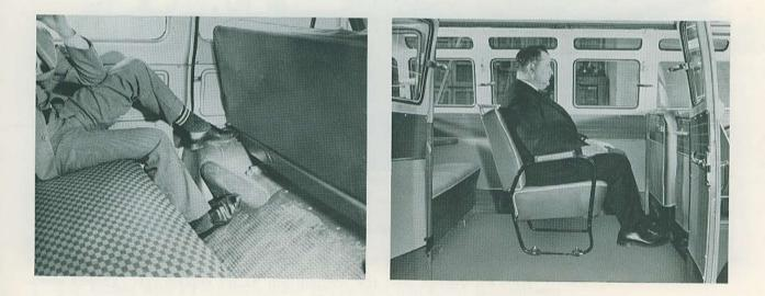
Our station wagon offers plenty of legroom, uninterrupted by wheel housing, or gas filler pipe, as in the Greenbrier. Notice the back of the Greenbrier's front seat. At 3,000 miles, the seat cushion has badly sagged and the springs show through the backrest upholstery.
