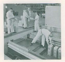
The Volkswagen is just as easily loaded or unloaded from sides or rear. The Chevrolet tailgate does not drop down vertically, making loading and unloading awkward, and preventing the vehicle from being backed up flush against a loading dock. Also note, that the VW Pick-up bed is much closer to the height of the standard loading dock, particularly convenient for farmers and tradesmen who regularly pick up and deliver at truck terminals.
