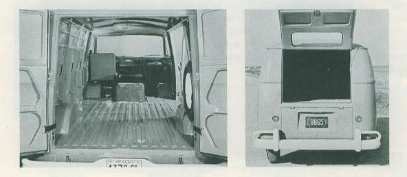
The Econoline's rear entry, 25 inches from the ground, offers somewhat easier loading from street level than the VW Panel, while dock-loading the VW Panel is relatively easier than on the Ford Van. Placement of the spare tire within the Ford Van necessitates unloading the truck to change a flat. In spite of similar loading space volume, the VW's payload capacity exceeds the Econoline Van by 930 lbs.
