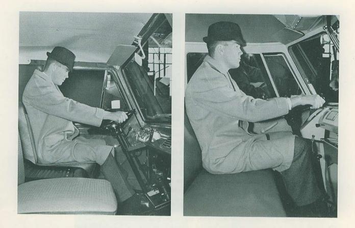
Headroom, a pain in the neck if you don't have it, as evidenced in the Ford picture, is clearly superior by two inches in the Volkswagen. The VW driver has plenty of room for his left arm compared to the cramped quarters of the Ford. A natural relaxed driving position is further aided in the VW by the almost horizontal steering wheel. The passenger seat is a \$35.40 extra on the Ford.
