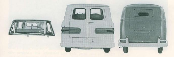
An annoyance feature on the Corvan is the rear windows, split by a door post that obstructs vision, making it difficult to see to the rear. Rear bumper guards and overriders are not available on the Corvan. Quality again—notice the difference in the way the Chevrolet doors fit; there is a minimum of space around the VW doors, while on the Corvan, space surrounding the doors permits snow, rain and wind to enter the vehicle.
