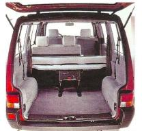
Not only has the engine compartment been kept very small due to the space-saving transverse installation of the engine - something from which interior space profits. The front and rear axle have also been arranged so that nothing is in the way in the interior. And loading is easy with the low loading surface and large tailgate.
