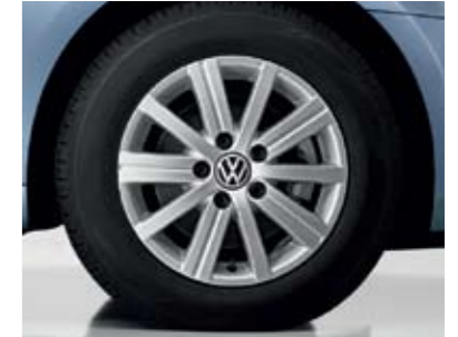
'Wellington' 6½ x 15 light alloy wheels with 195/65 R15 tyres. Optional on S models.
