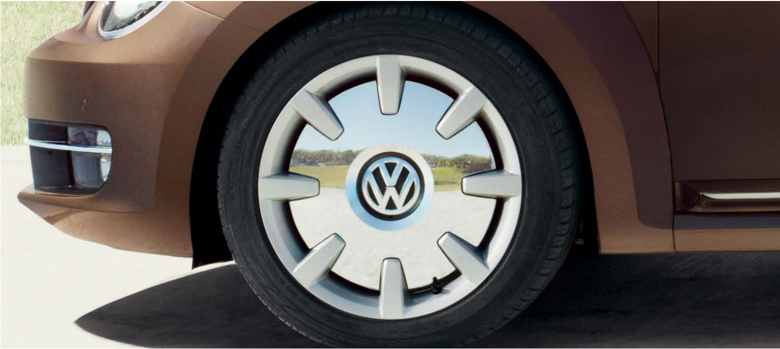
18 inch 'Discus' alloy wheels with 235/45 R18 tyres and anti-theft wheel bolts. D SP (No cost option on Sport models.) Image shown is Beetle Cabriolet Sport with optional Bi-xenon headlights and metallic paint.
