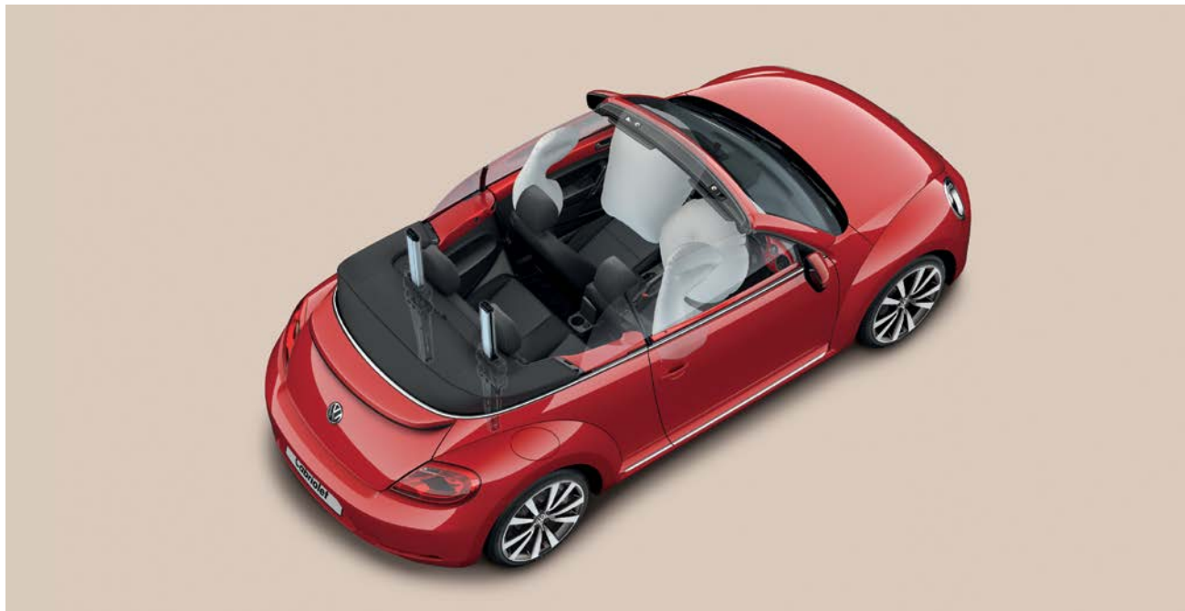
There is no compromise in safety with the Beetle Cabriolet's comprehensive airbag system . Included as standard are driver's and front passenger's airbags, with a front passenger's airbag deactivation switch and driver's and front passenger's combined head and side airbag system.
