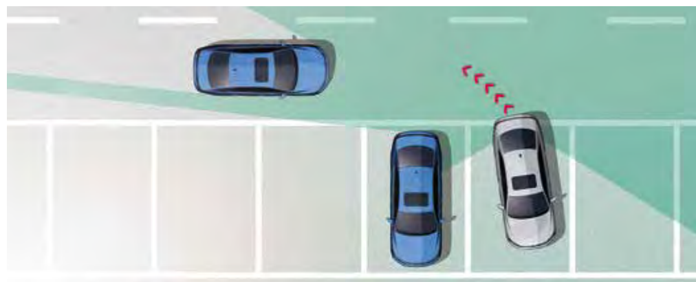
The parking sensor pack comprises front and rear parking sensors and reverse activated kerb-view adjustment on the passenger's side door mirror. The parking sensors assist in parking manoeuvres by emitting ultrasonic, audible and visual signals, alerting the driver to any obstacles in the way. In addition, an optical parking display extends the functions of the parking sensors by indicating your position, either on the RCD 510 radio system (Optional on Trendline, standard on Comfortline and Highline) or the RNS 510 radio system (Optional on Trendline, Comfortline and Highline), on the vehicle's audio display during parking.
