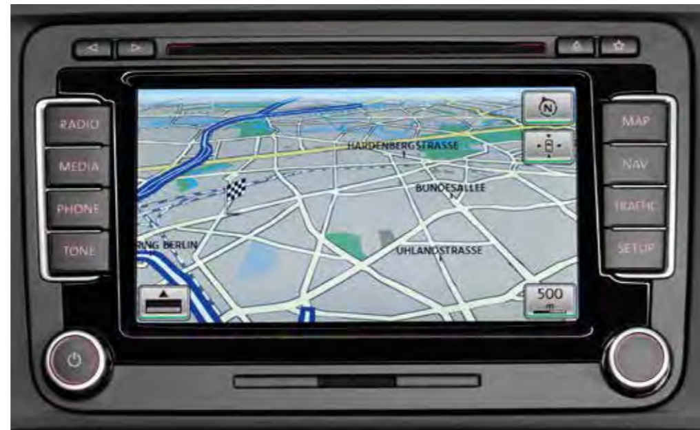
Radio/Satellite Navigation RNS 510 SatNav with TFT Display, touch screen, 30-GB hard disk, SD card reader and DVD drive.
