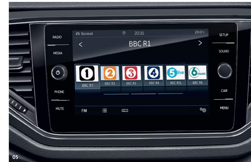
05 The Composition Media infotainment system is equipped with an 8.0 inch colour touch-screen, DAB digital radio receiver, Multi Device Interface (MDI), single CD player, SD card reader and USB connection. It allows music playback from MP3, WMA and AAC files, simultaneous pairing of two compatible mobile devices, SMS functionality (when stationary and on compatible Android smartphones only), Bluetooth telephone and audio functionality 1 , and provides driver tips and journey analysis via the 'Think Blue. Trainer.' Six speakers, situated to the front and rear, make sure excellent acoustics are delivered on every journey.
