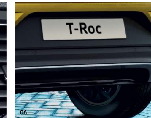
06 Front and rear parking sensors assist parking manoeuvres by emitting both audible and visual signals, alerting the driver to any obstacles in the way. The closer you are to an obstacle the faster the sound frequency, while an optical parking display indicates your position in relation to obstacles on the screen of the vehicle's infotainment system. Standard on SE and optional on S models.
