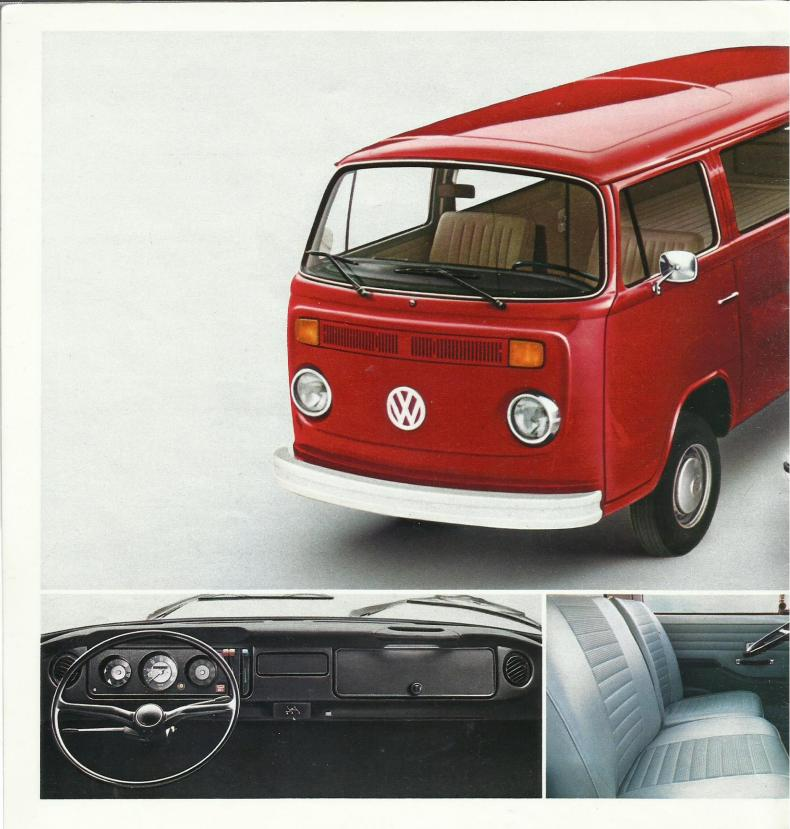
This seven, eight or nine-seater from VW has a great deal in common with a saloon. And with its 178.9 ins. of length (4545 mm) it fits as easily into the same parking space. While with its 69.3 ins. (1760 mm) it also goes into any standard garage. Or take its semitrailing arm axle that gives it its good roadholding characteristics. Or the 1700 cc engine and twin carburettor. And automatic transmission, too — hitherto a special privilege reserved to passenger saloons.
