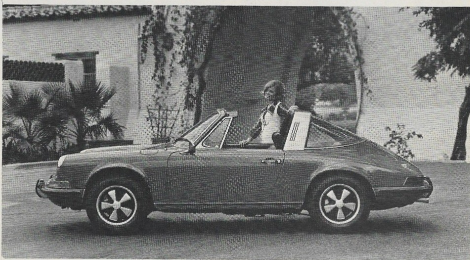
The "Targa" convertible is the optional body style with its built-in roll bar and stowable top. It's newly available with any of the engines.
