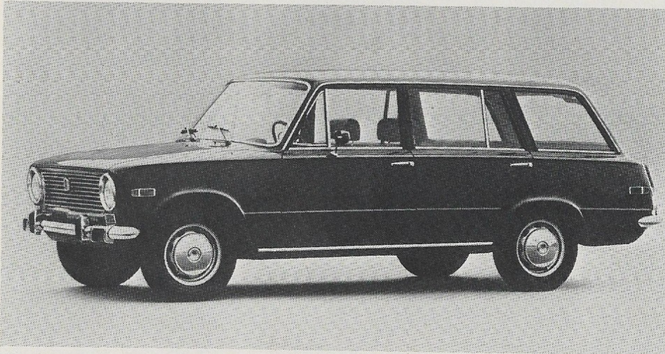
Though not shown, a chrome roof rack is standard on the 124 wagon. The 76-hp engine is front-mounted and there's servo-assisted disc braking at four wheels.
