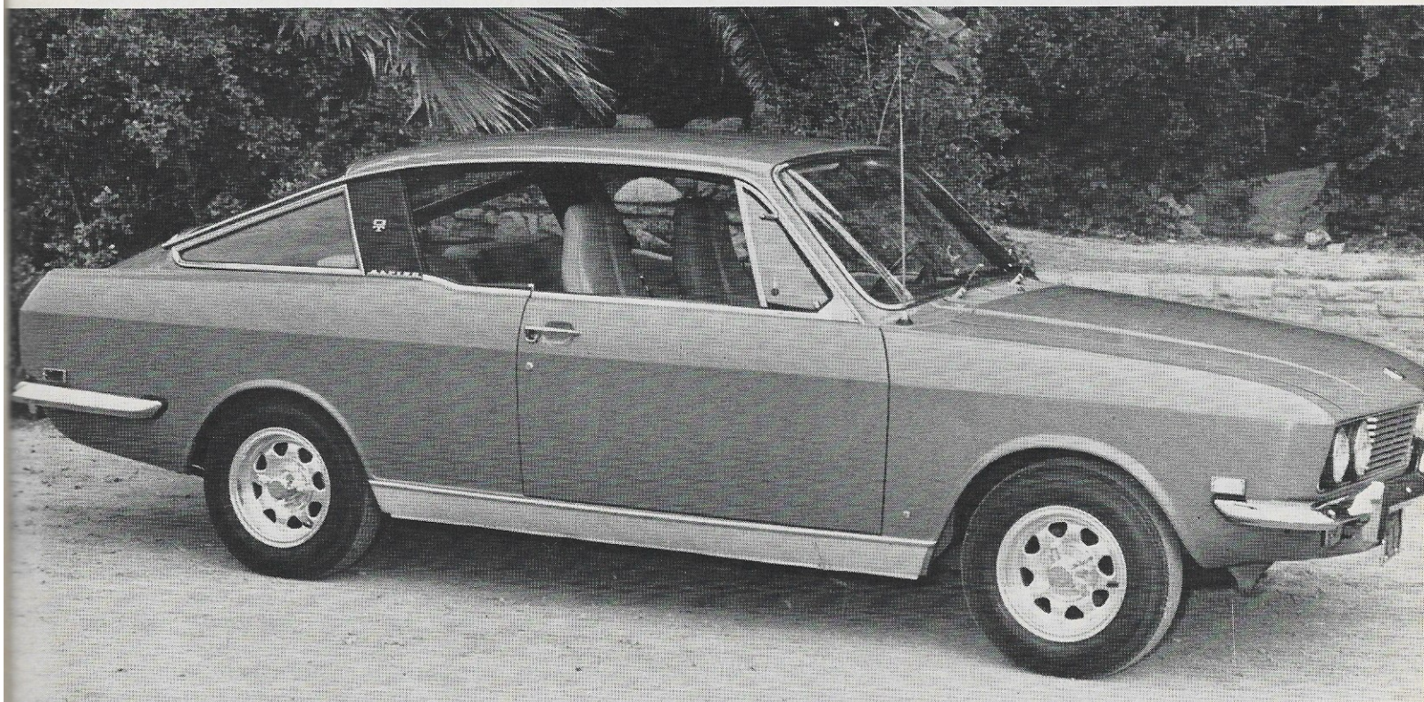
Towering buckets don't help rear vision much but comply with U.S. safety regulations. Wrap-around bumpers adequately protect the car in parking lots.
