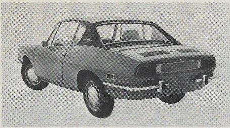
Sleek 850 Sport Racer is Bertone's latest contribution to Fiat's U.S. offerings. Vents in roof are part of the flow-through ventilations system.
