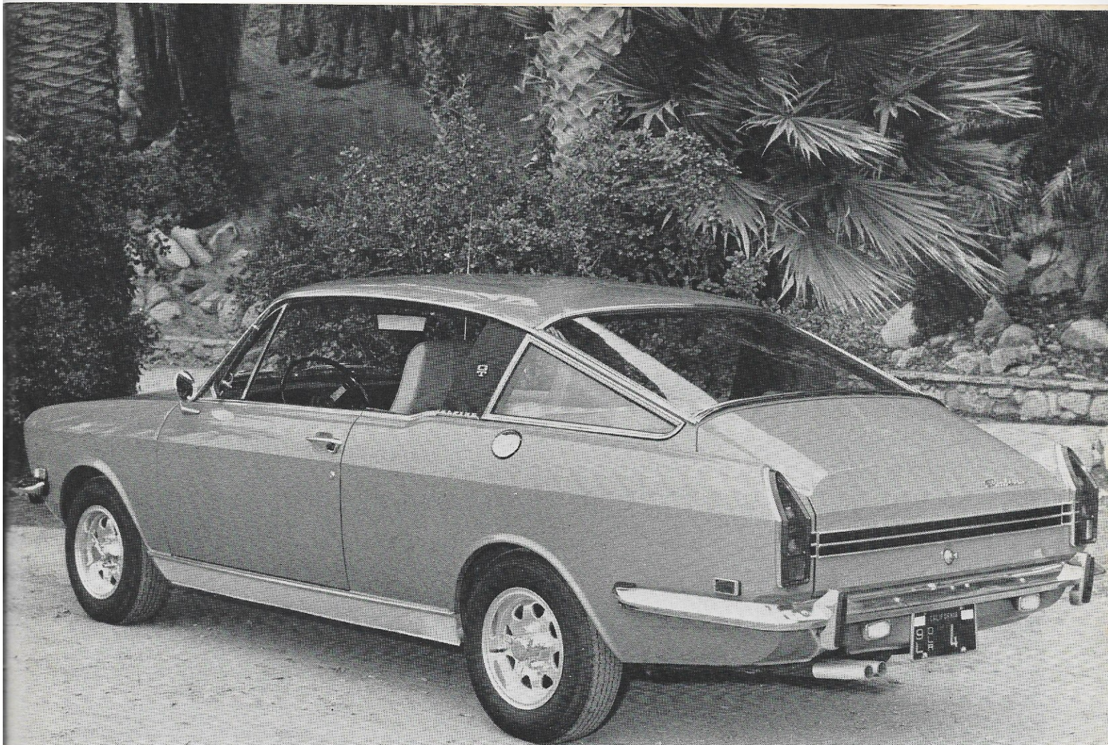
Dual exhaust outlets are just an extension from the resonator. Nice-looking "mags" are a Bud Shroeder design carried over from the original Alpine V-8.
