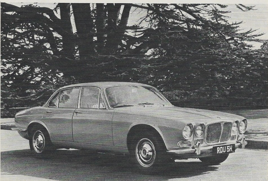
Integral body/frame construction is on a suspension tuned for Dunlop's new radials with a unique "anti-aquaplaning" tread. Car meets U.S. emission and safety requirements but won't be officially imported.
