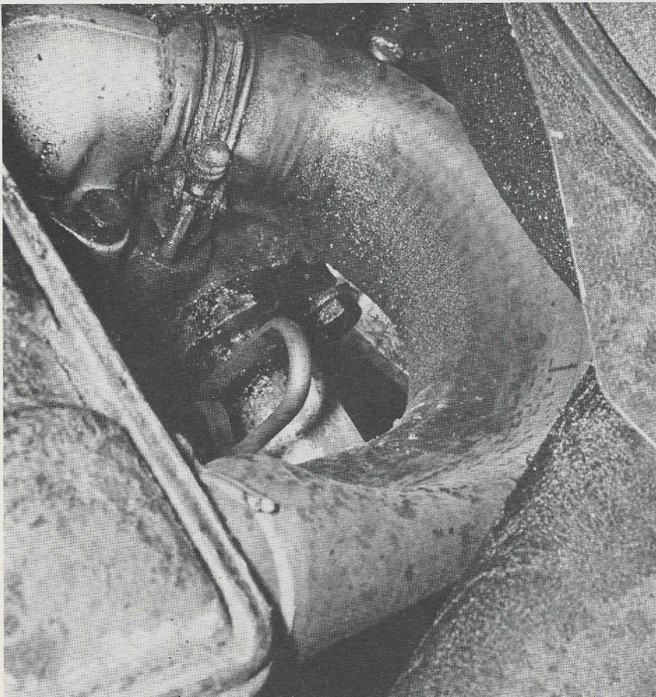
Collapsed and flattened hoses such as this can restrict coolant circulation and cause severe overheating. They may soon burst under pressure also.
