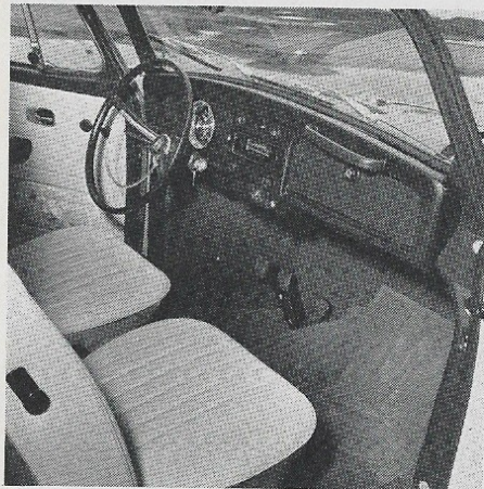
Instrumentation and trim is carryover. Large ignition key which locks the wheel is still sometimes difficult to insert.
