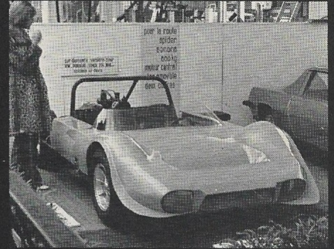
The Belgian Mean (pronounced mee-ann) is a $750 fiberglass kit in coupe (right) and roadster form that takes VW, Porsche, Simca, BLMC etc. running gear.
