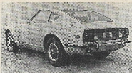
Rubber imbedded bumper wraparounds are a neat touch as is the lockable antenna for the standard radio. Tailgate glass has an imbedded heater.
