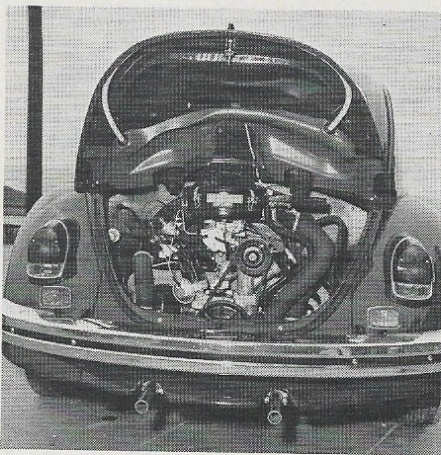
Vulnerable Porsche-like reflectors are a '70 addition, as are the tubes to drain water that might seep in from the slots in the engine lid.
