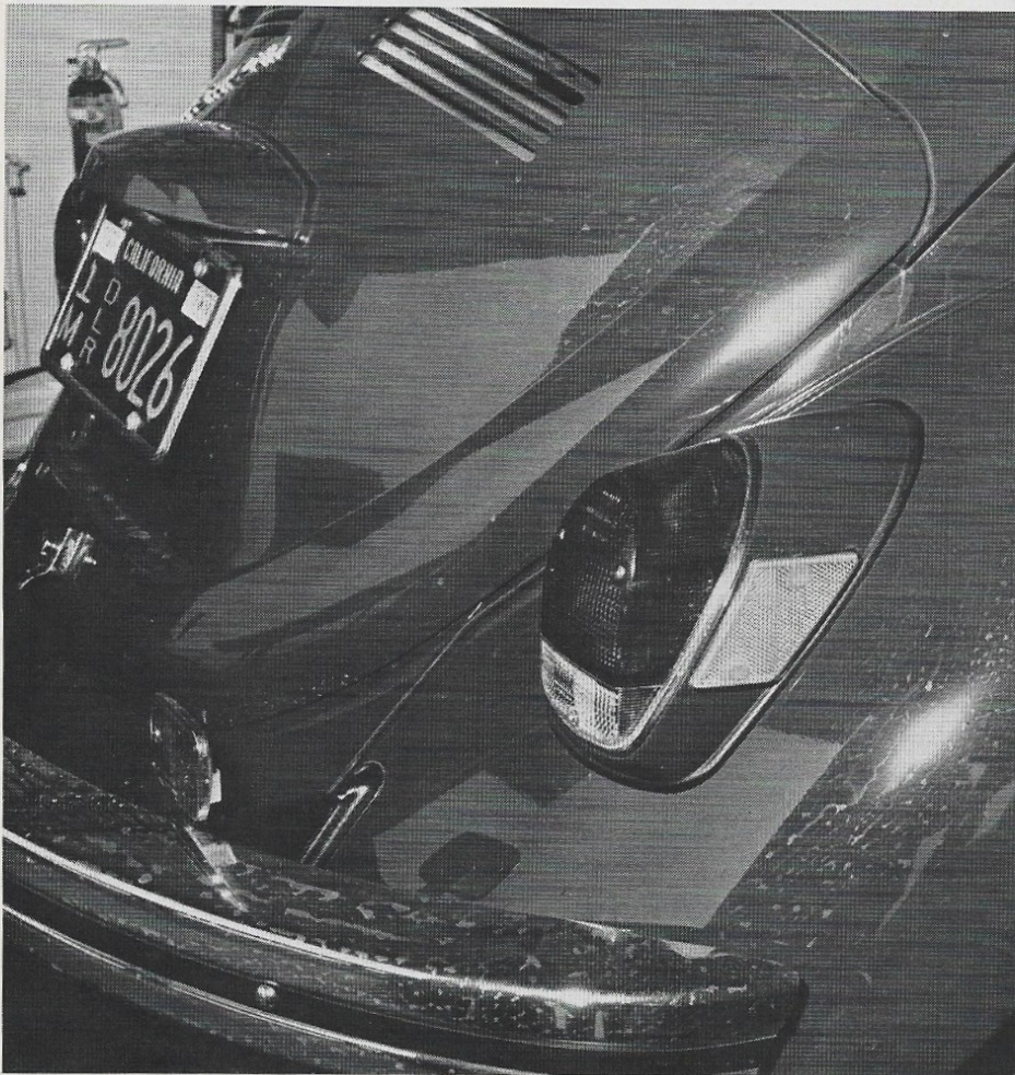
The new slots in the engine lid are essentially the same as used on the convertible but may affect usage of luggage racks. No advice is available on this.
