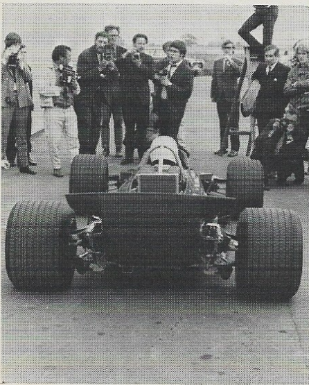
Integral aerofoil also acts as an effective fairing for the rear drive components, the front being left open to the breeze. Unlike Indianapolis, there is no thought of banning all-wheel-drive in Formula 1.
