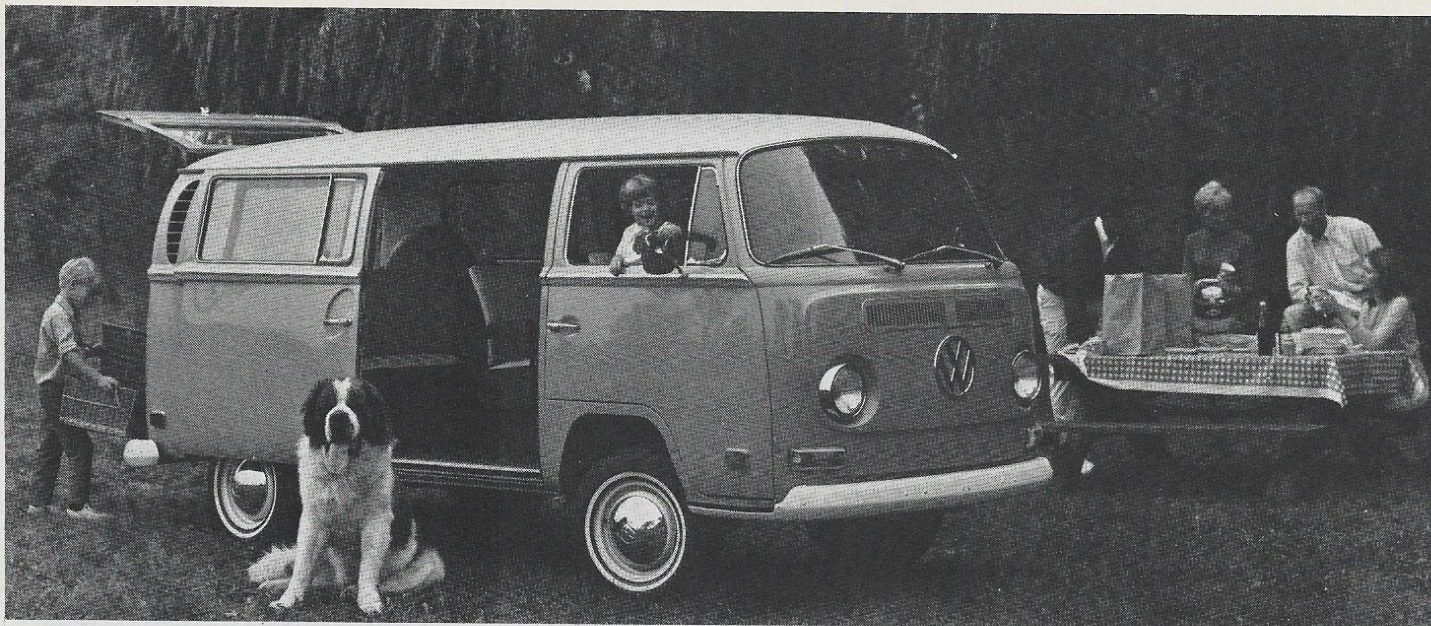
1970 wagon may be identified by reflectors added to each corner. Except for minor carburetion modifications, the 1600-cc engine with 57 hp remains the same.
