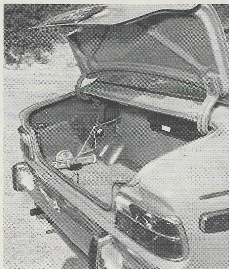
Jack stowage and sharp edges in the commodious trunk could wreck some havoc with fine luggage but the area is dust and wet proof.
