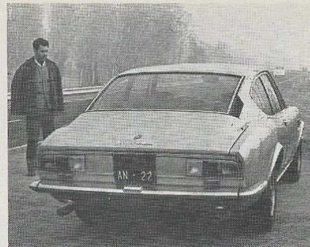
Rear view shows the clean, functional lines to advantage. Vents at the rear window serve the flow-through ventilating system.
