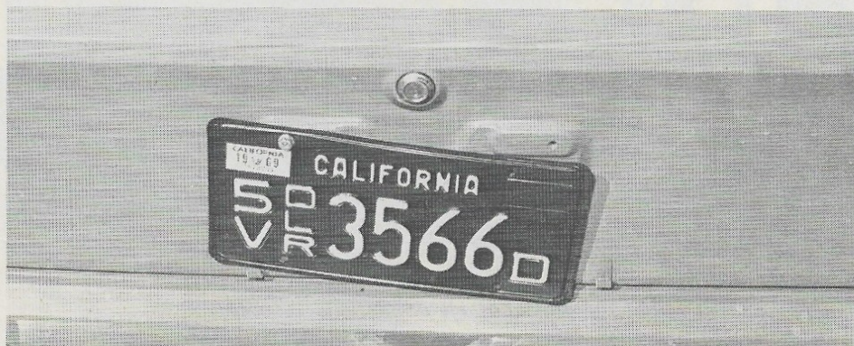
Oddly enough the raised and drilled plate escutcheons at the Corollas rear do not fit the standardized U.S. plate.
