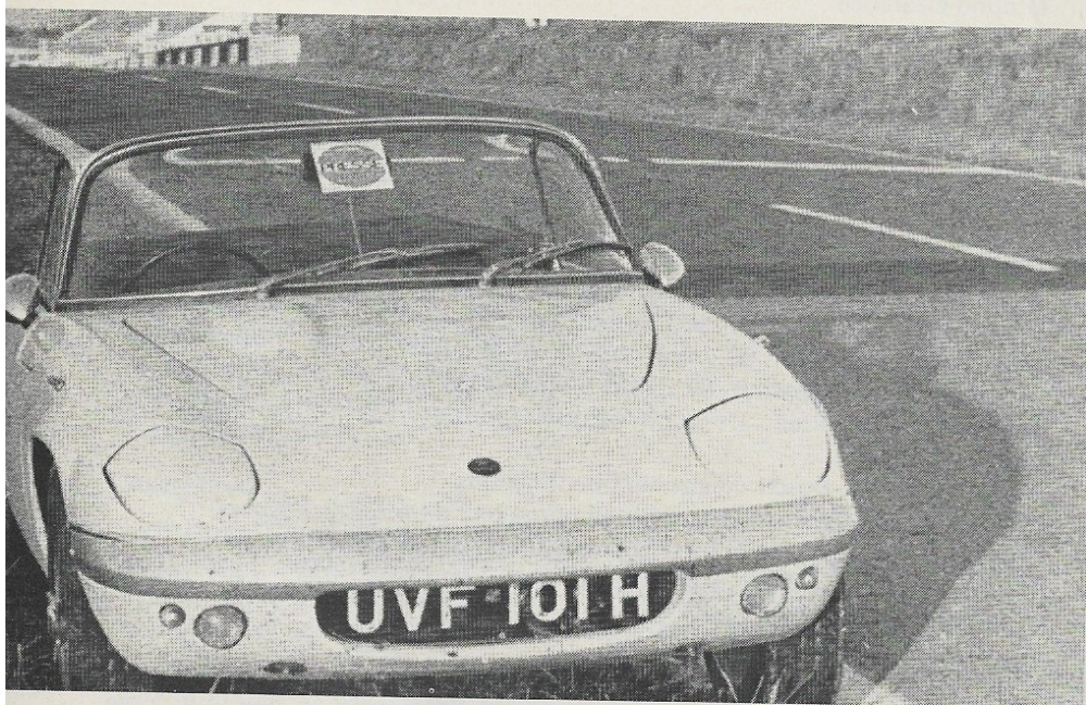
Dual carburetion requires a hump in the hood for clearance. Tiny radiator causes cooling problems under severe conditions, despite electrically driven fan.
