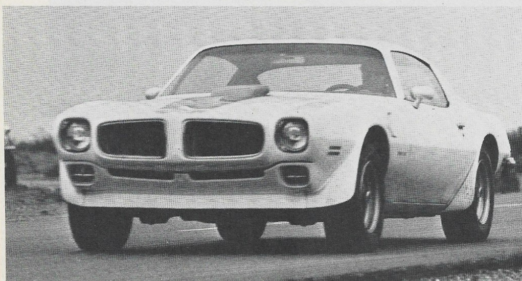
Ram-air intake for the Trans Am emerges through a hole in the hood. Brittle ABS plastic spoiler in front is aerodynamically efficient but vulnerable to curb damage.
