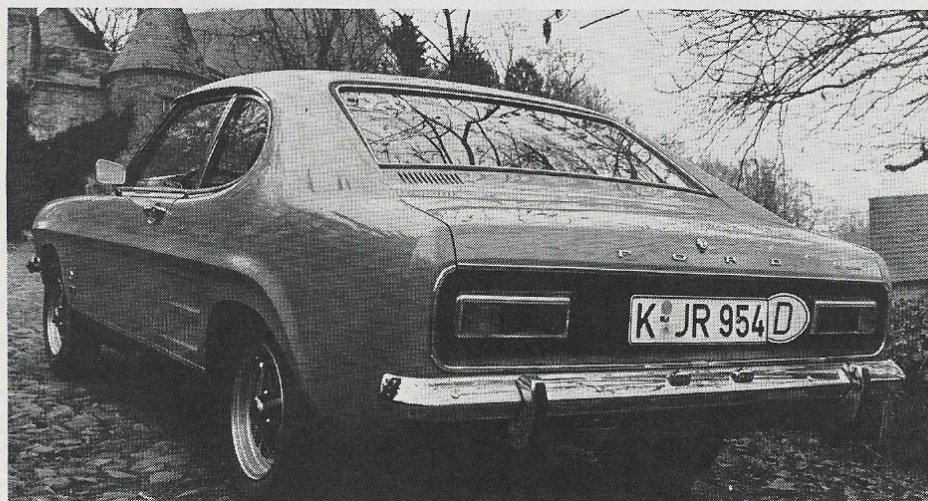
Modern full-flow ventilation, as evidenced by the vents in the deck, is built into every Capri. It will carry four in reasonable comfort.
