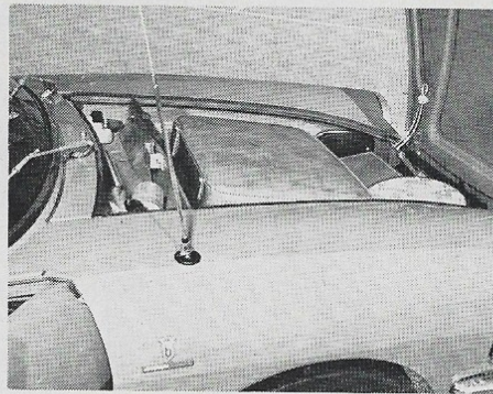
Luggage space in front is minimal but adequate gear for two may be carried inside the car. Note the simple but positive catch to hold the lid open.
