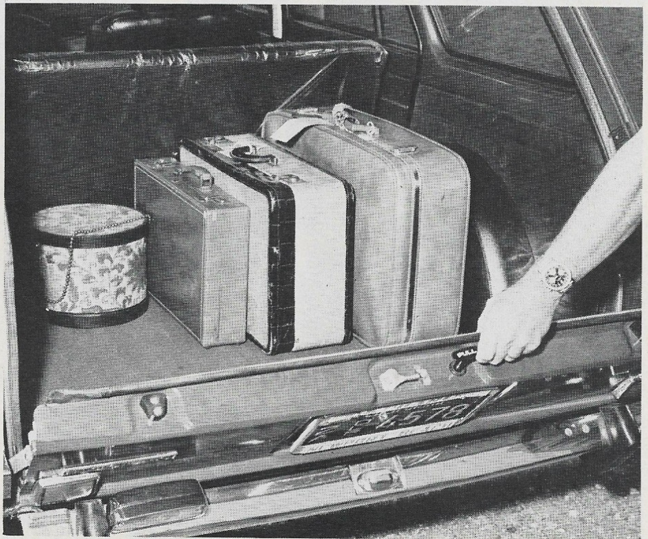
Tailgate is formed from two sections, resulting in a few rattles. Ingenious divided bumper, fuel tank under the rear seat and spare in the engine compartment permits unusually low gargo floor.
