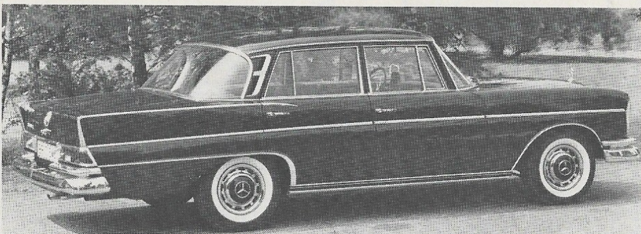
After the discontinuance of the 300 D limousine in 1963, the three-liter, injected, 180-hp engine was adapted to an upgraded 220 Series chassis and the body called the 300 SE.
