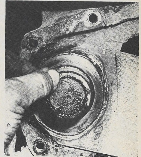
Torsion bars are marked "L" and "R" for left and right. Don't mix them. Mark on hub can be in line with bend in letter "L" or one leg of the letter "R". (Note comment
