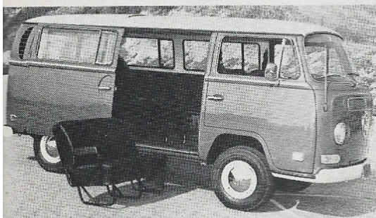
The middle seat unbolts in minutes and the lugs themselves slide right out to gain a flat loading floor for bulky cargo.
