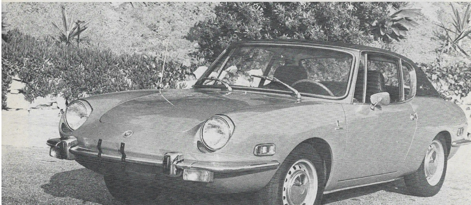
Front end, including license plate, sheetmetal and parking lights is rather vulnerable to damage from careless parkers and high curbs.
