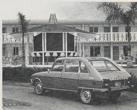
C. Entire back end above the taillights swings up to form a fifth door. Ridges in roof are for structural strength, not to improve aerodynamics.
