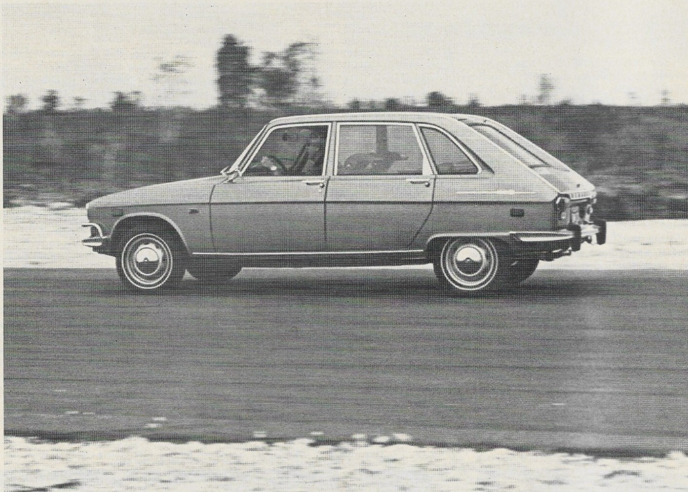
A. Only evidence of a full-throttle acceleration given by the Renault 16 is that the rear squats down to a more normally level position. You can't spin the front wheels.
