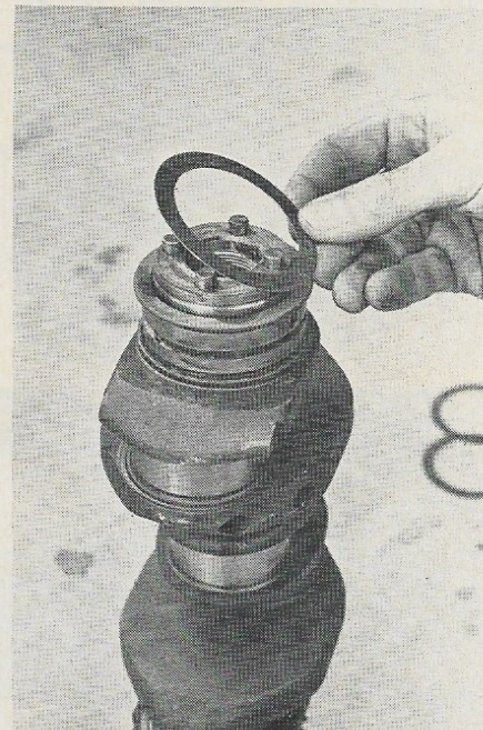
B. Crankshaft shims should be saved for use in re-assembly. Fig. 2
