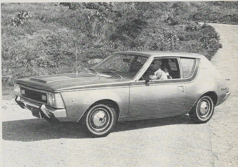
B. Front sheetmetal of the Gremlin is shared with the larger Hornet, saving millions in tooling costs and permitting use of interchangeable engines and running gear.
