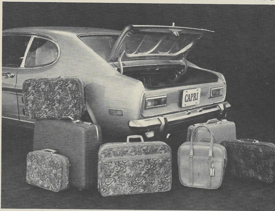
Presumably all this can be carried in the Capri's 7.2 cubic foot luggage compartment. Note position of the gas tank well inside the trunk area.
