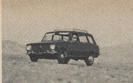
Panic stop with brakes near locking point produces only very moderate nose diving. Disc brakes are smooth and even under all circumstances.
