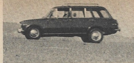
Panic stop with brakes near locking point produces only very moderate nose diving. Disc brakes are smooth and even under all circumstances.
