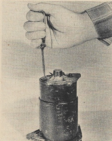
All generators come apart the same way. Remove the two long screws that hold the ends together. Most brush replacements must be done this way.
