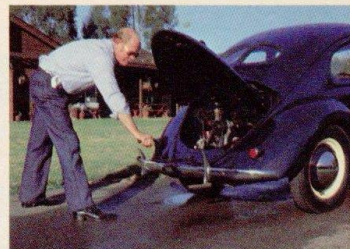
Karl Belcher demonstrates how to crank a beetle. More than two decades have passed since VW came equipped with a “handle.” (Vince Manocchi photo)
