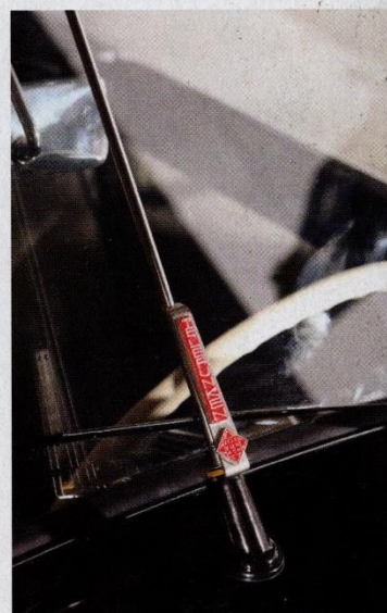
Ultra cool and rare Telefunken center-mount radio antenna keeps the tunes crisp.
