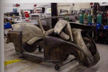
The Hebmüller's shell post acid dip at Metal-Works Paint & Rust Removal.
