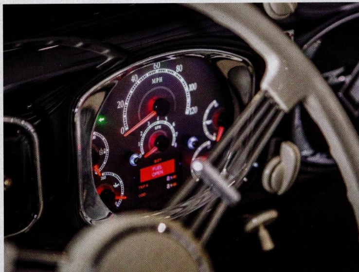
Monitoring the vitals is a custom-built set of Dakota Digital HDX gauges that fit perfectly in the early dash pod. The one-off set was built off early Bronco gauges.
