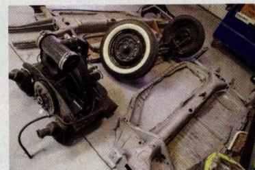
Both the stock and 1970 IRS pans in pre-restoration condition.
