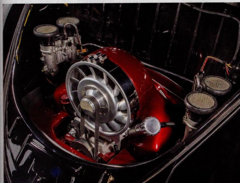
Body color-matched "Blood Red" Bernie Bergmann fan shroud and dual Weber 48IDA carbs make for a clean and sexy engine bay.
