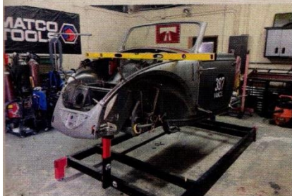
Thanks to a second jig used to mount the windshield, the crew could fit other panels.
