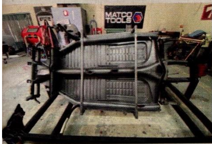
After fixing the severely rusted and damaged tunnel, the team spot welded in new pan halves.
