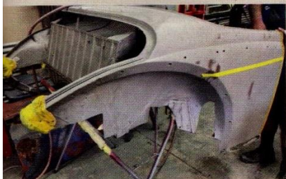
In many areas, the remaining metal was extremely thin, measuring 28 gauges.
