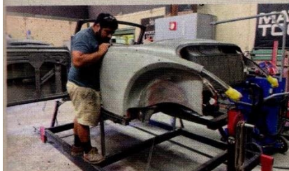
Mocking up the rear quarter panels in great shape... The '49 sedan supplied these pieces.
