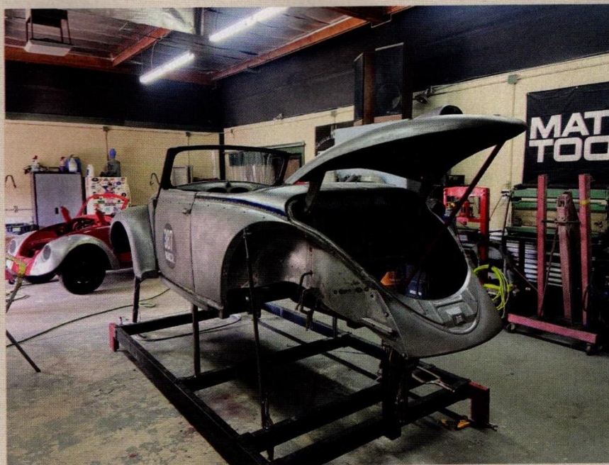
The decklid was usable, though it required many hours of straightening and massaging. Help from the Heb Hunters proved invaluable during the seven-month restoration.
