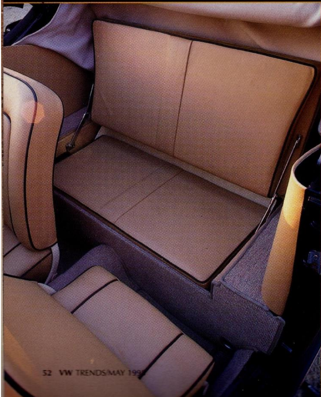
LEFT and BELOW: Octavio Gutierrez re-covered the repainted seat frames using Biscuit Reno-colored leather with black piping.
