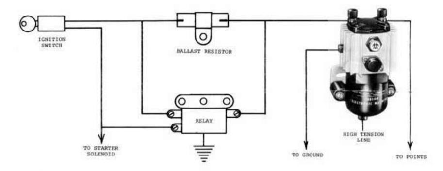
On automotive engines use Delco ballast resistor No. 1957154 which can be purchased at any General Motors dealer. Marine engines use Mopar ballast resistor No. 2444142 which can be purchased at your Chrysler marine engine dealer. Ballast resistor can be fastened to the magneto mounting plate with one of the mounting screws. Ballast resistors become very hot in operation and should be kept clear of wires and hoses.
