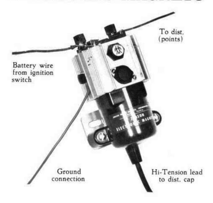
Same unit is used on both 6 volt and 12 volt systems. Installation procedure is exactly the same for both negative ground and positive ground systems. The difference is in the magneto itself, not its connection. Do not install a standard negative ground unit on an engine having a positive ground. Units for positive ground systems as required on British engines and some American engines manufactured prior to 1956 are stamped on the front "positive ground".
