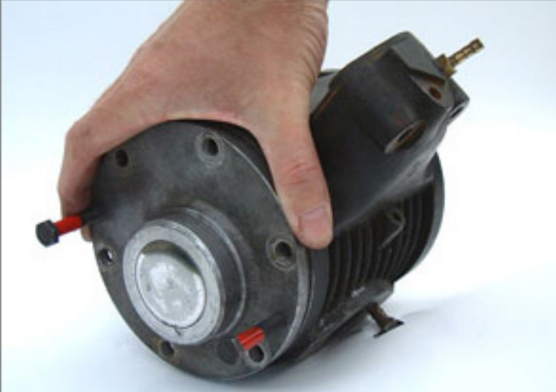
Use two 5/16th USS bolts to remove rear cover
