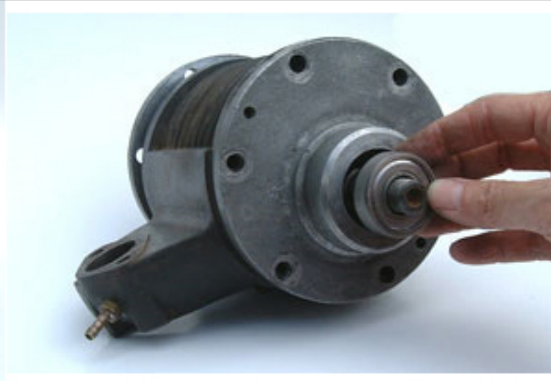
The main bearing fits snugly into the front housing
