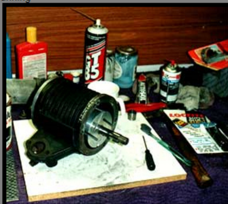
The rotor has been dynamically balanced for smooth running
