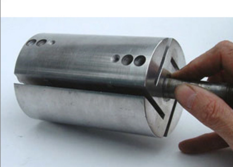
Use two 5/16th USS bolts to remove rear cover
