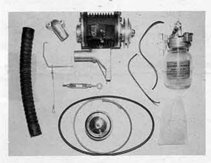
Here is a complete supercharger installation designed specifically for the Renault Dauphine. Everything is furnished with the kit and the installation can be made easily with standard tools in less than two hours by following the illustrated instructions furnished with the supercharger.
