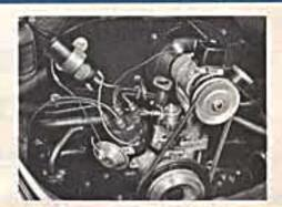
Replace studs and jet in carburetor, fasten carburetor to supercharger and connect throttle linkage. Illustration shows supercharger and carburetor as used on Volkswagen engines manufactured prior to 1961.
