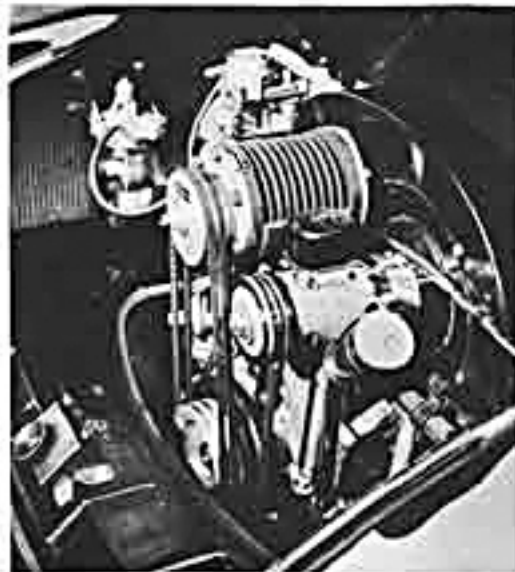
The Judson vane type compressor installed using a stock 28 PCI carburetor. The little Ghia coupe accelerated from 0-60 in 15 seconds, half of stock time.
