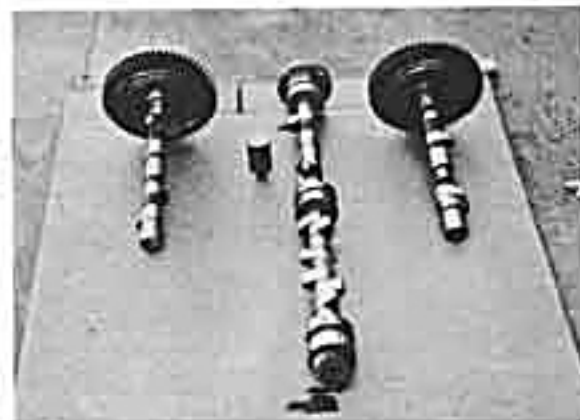
Semi-race cam on left, Iskenderian "401" with radiused tappet in the center, and full race grind on the right. The "401" grind forms basis for VW cams.
