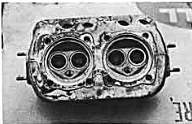
Stock head shows small sized valves. Any possible gain made by the installation of larger valves is effectively nullified by barrel spigots which cannot be relieved.
