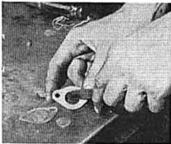
3 Block carburetor heat riser by reaming out gasket with knife and inserting pennies in resulting hole. Blower creates own warmth.
