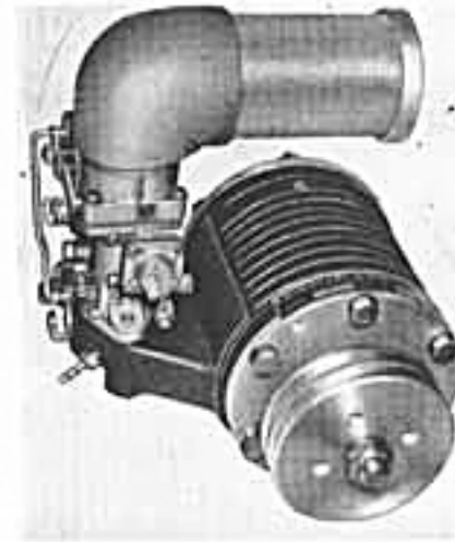
For VW, Judson supercharger uses stock carburetor with an unusual air cleaner.
