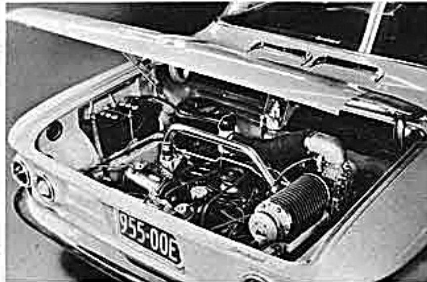
Judson supercharger installation on Chev Corvair rear engine. Uses special crossover pipe to opposite bank, with larger 2-throat carb.
