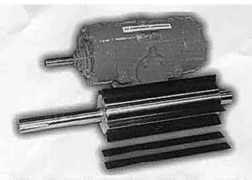
■ The Torlon 7130 vanes, shown next to the rotating element, are extruded "on-size" by a special process developed by Drake Plastics, and then precision cut to meet the OEM's specifications. Torlon 7130 and 4301 resins are produced by BP Amoco Chemicals, Atlanta, Georgia. The Torlon vanes provide three times longer wear than do the current asbestos-laminate vanes.
