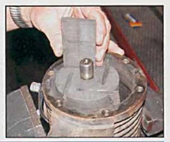
ABOVE, remove the six bolts that hold the back cover on. Remember, these are SAE threads, not metric. ABOVE CENTER, using two 5/16-inch bolts, screw them into the back cover and use them as jacking screws to pry the rear cover off the rotor shaft. ABOVE RIGHT, you can now pull the vanes out of the rotor, paying particular attention to the way they were installed.
