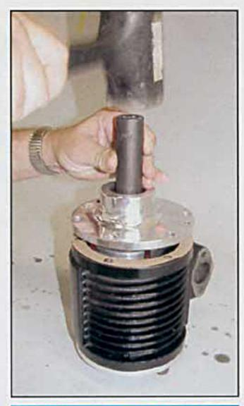
ABOVE, after placing the new gasket on the blower housing, locate a deep socket that fits over the rotor shaft that is the same outside diameter as the bearing, and press the bearing and cover onto the housing. Make sure everything goes on straight.
