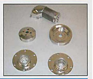
ABOVE, after having the blower case lightly honed, and the end plates machined to get them flat again, they were ready for reassembly. ABOVE CENTER, the blower case received a quick shot of high-temp spray paint. ABOVE RIGHT, the aluminum pieces were taken to Mag Masters, in Santa Ana, CA, where they worked their polishing magic on them. What a difference!
