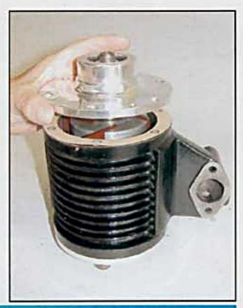
ABOVE, with the rear cover snugged down, but not tight, place the front cover over the rotor shaft. ABOVE RIGHT, make sure you don't tear the two seals in the front cover when you slide the cover onto the rotor shaft.
