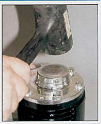
ABOVE, bolt down the rear cover, and check to make sure the rotor and vanes still spin freely in the housing. If not, find out where the binding is, either on the front or rear (or even both) ends, and shim with a gasket until the desired clearance is achieved. ABOVE RIGHT, when everything is tightened down, and still spinning easily, reinstall the plug in the rear cover. BELOW, the finished product.
