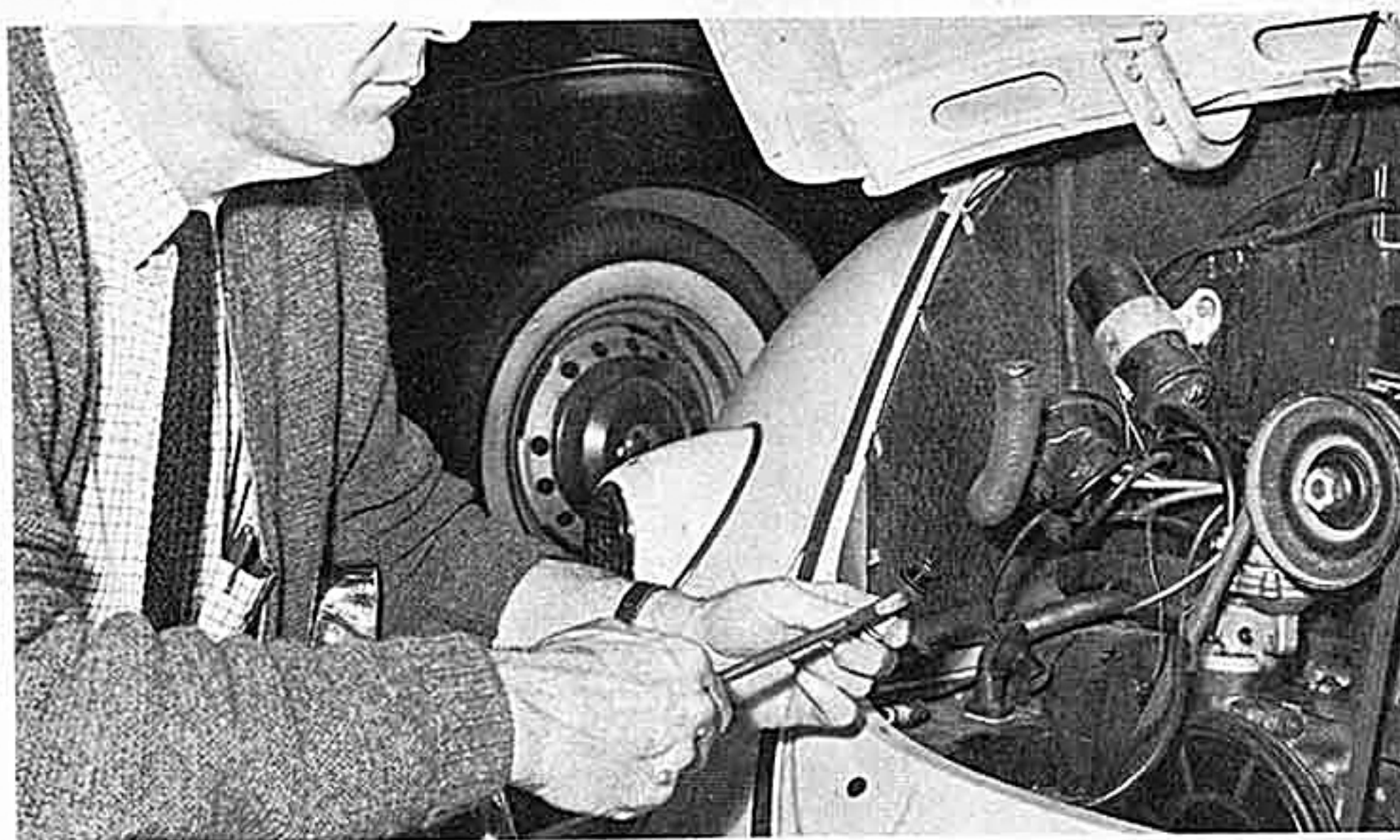
Judson distributor and supercharger expert Bill Corey examines sparkplug to determine if mixture is correct. Precision tuneup is important part of supercharger installation.
