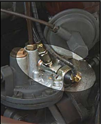
Outlet from the crankcase is through a "T" piece screwed into the oil pressure outlet.
