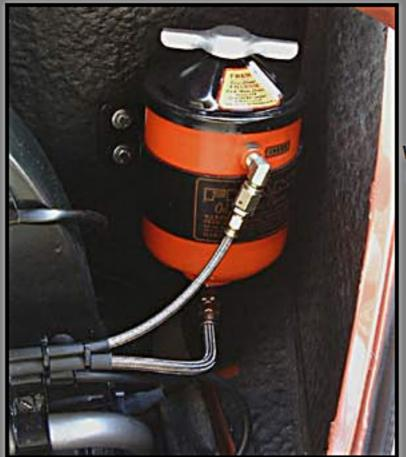
With a Judson Supercharger and Marvel Oiler in place there is only one obvious location for the Fram Oil Filter, on the right hand side of the engine bay attached to the firewall.
