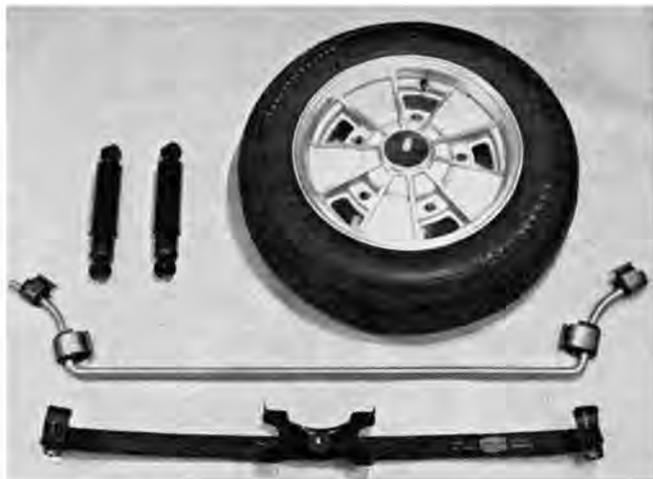
**HANDLING PACKAGE** includes camber compensator, heavy duty shock absorbers, anti-roll bar, special wheels and tires.
