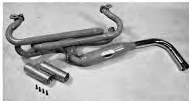
**EXTRACTOR EXHAUST** systems for VWs are manufactured by Cyclone, Bursch and EMPI (above). Prices are near \$50.
