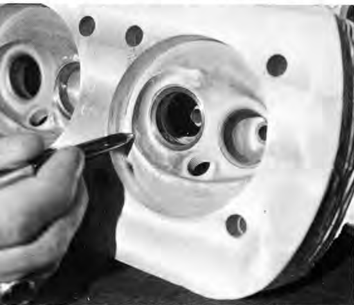
Revmaster reworks the combustion area to improve the engine's breathing capacity. In the process the chamber is shaped to avoid detonation which can be a problem with high compression VW engines.
