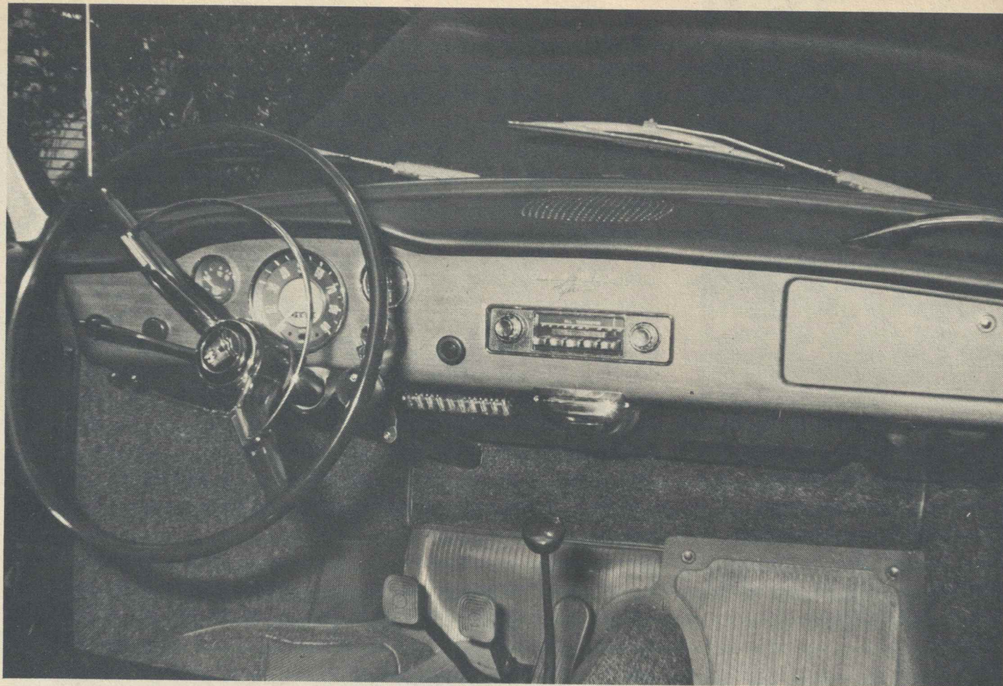
ABOVE: Smaller clock and gas gauge with warning lights are the big changes.
