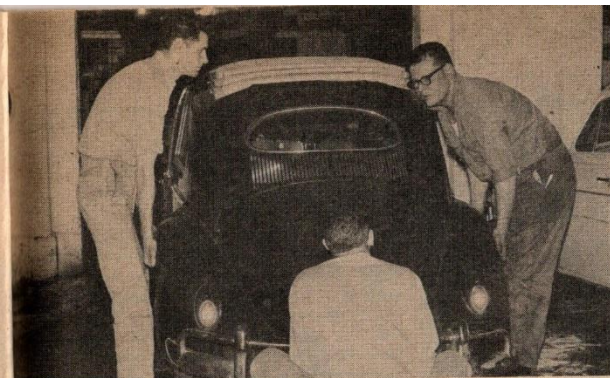
Left: One way of swapping is to use three stout men at each end and lift. Below: With body firmly supported, the chassis may be removed by using a roller jack or dolly. Bottom: A hydraulic lift may be used and then roll out happily.
