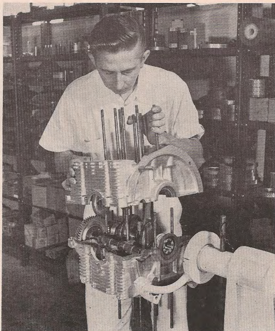
Horvath fits the two VW magnesium crankcase halves together. VW cases and bearings have proven quite capable of absorbing added load of a modified engine without giving any problems but Joe installs heavy-duty steel-backed main bearings to be safe.
