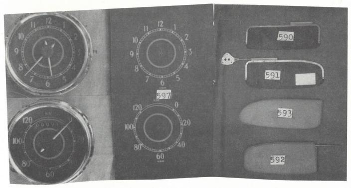
597 Speedo and clock faces, silkscreened on gummed vinyl by the So. Calif. VDO shop. Both the speedo and clock above have had the new faces applied. Since the hands and pointer are difficult to remove, we suggest that application be done by a speedo shop. Each for \$9.00. Both faces for - -
