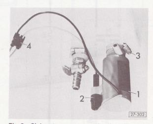
Fig. 5 Sink water pump, removing/installing
