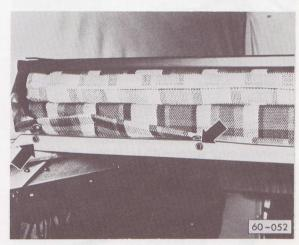
pull off double bed snaps (arrows) at frame and remove mattress
