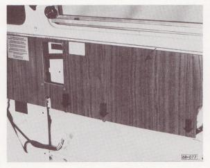
remove Phillips screws (arrows) and pull trim panel out of channel
