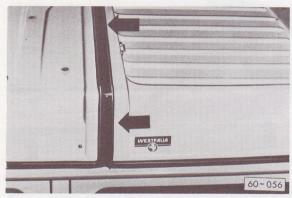
check alignment of pop-up roof to luggage rack and seating of seal (arrows)
