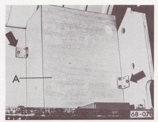
remove Phillips screws (arrows) and then cover for rectifier
