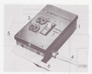
Fig. 2 Circuit breaker and auxiliary outlets
