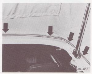
— remove screws (arrows) at channel
