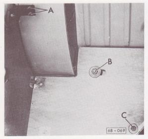
remove 2 self-locking nuts (A), nut from anchor bolt (B) and bolt from floor (C)
