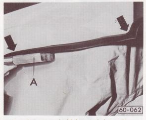
— to make sure seal with inserted clamps is seated properly on roof press it onto edges with plastic wedge (A)
