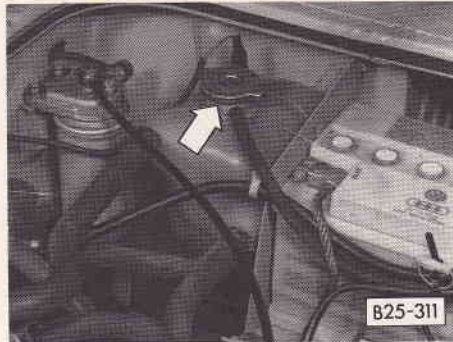
Expansion tank Diesel engine
