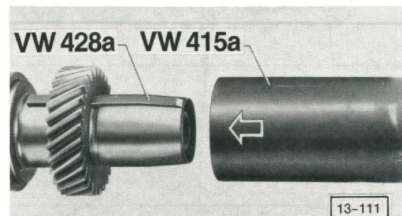
Fig. 5 Distributor drive gear/crankshaft timing gear, installing
