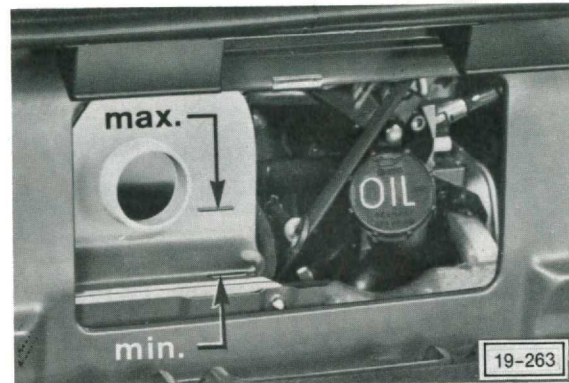
Fig. 8 Cooling system, filling
