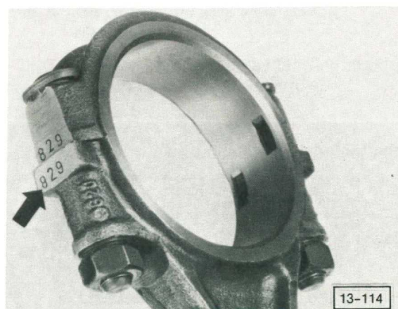
Fig. 6 Connecting rod, installing
