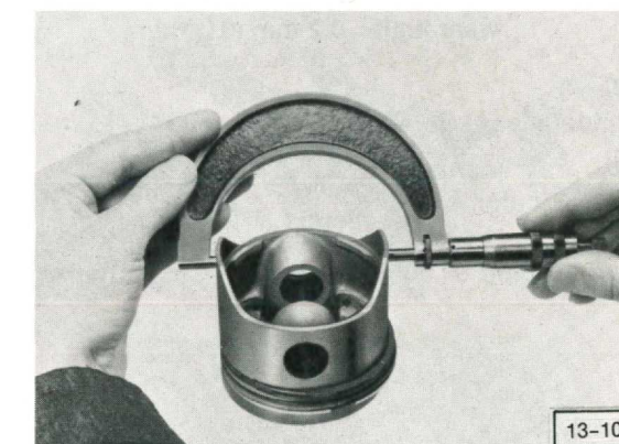
Fig. 9 Piston, checking diameter/wear
