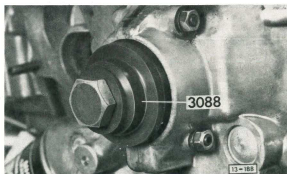
Fig. 6 Crankshaft oil seal, installing Single pulley — coat seal lips with oil and install seal with 3088 and pulley bolt (without washer) — then tighten bolt with washer until stop Triple pulley — coat seal lips with oil and install with 3088 and pulley bolt without washer and tighten bolt until stop
