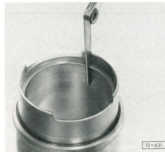
Fig. 7 Piston ring end gap, checking
