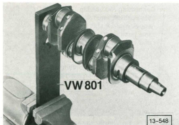
Fig. 1 Crankshaft, clamping in vise
