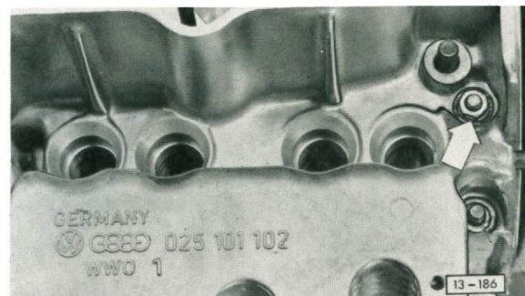
Fig. 4 Crankcase halves, assembling — first tighten M 8 nut (arrow) — then tighten all M 10 nuts — tighten remaining M 8 nuts
