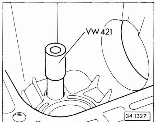
**Fig. 8 Driving needle bearing out of gearbox housing**
