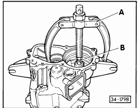
**Fig. 8 Removing needle bearing**
