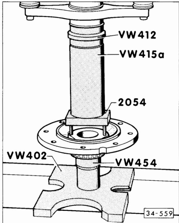
**Fig. 4 Pressing inner race/tapered roller bearing off cover**
