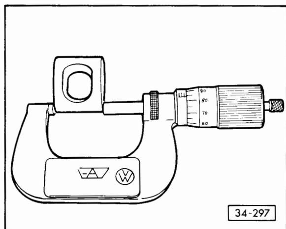
Measure the shortest spacer sleeve (Part No. 002 517 241) with a micrometer and mark the actual dimension on the sleeve with an electric marker or similar device. The sleeve should then always be used as a measuring sleeve and should be kept with the measuring device.
