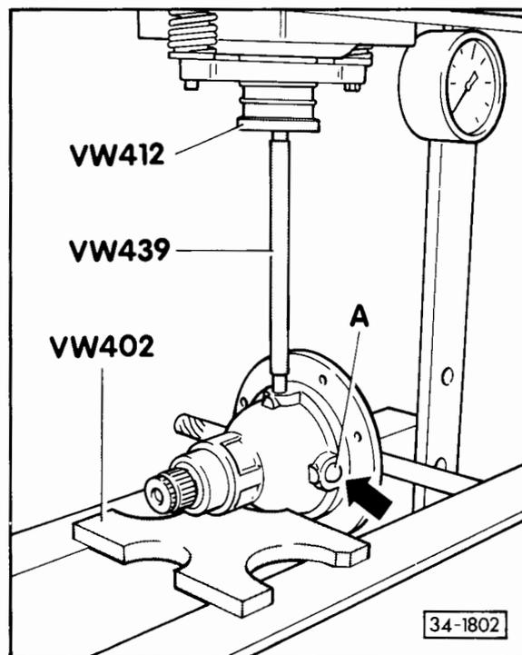
**Fig. 7 Pressing out differential pinion shafts (short)**
