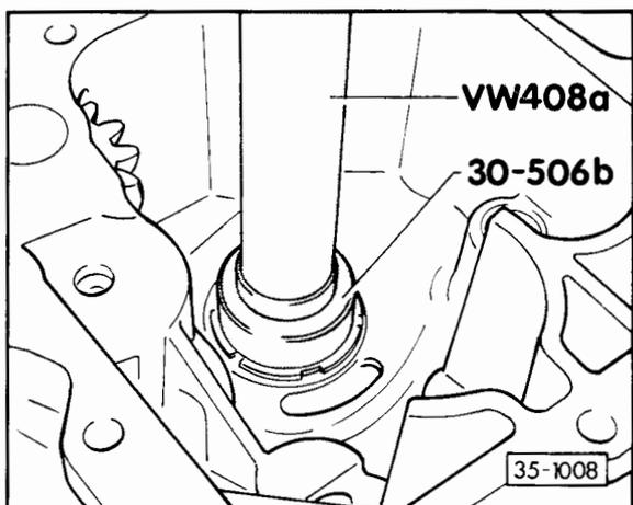
**Fig. 18 Pressing complete bearing into bearing carrier cover**
