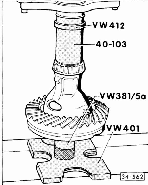
Fig. 11 Heat inner race of tapered roller bearing to about 100° C, install and press home
