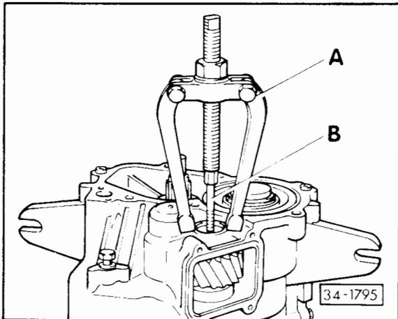
**Fig. 1 Removing idler gear for cross-country gear**
