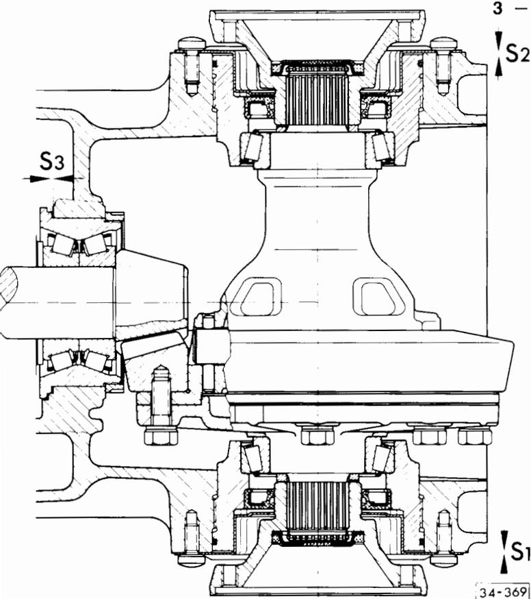
$S_1$  = Screw-in depth of adjusting ring (crown wheel end)
