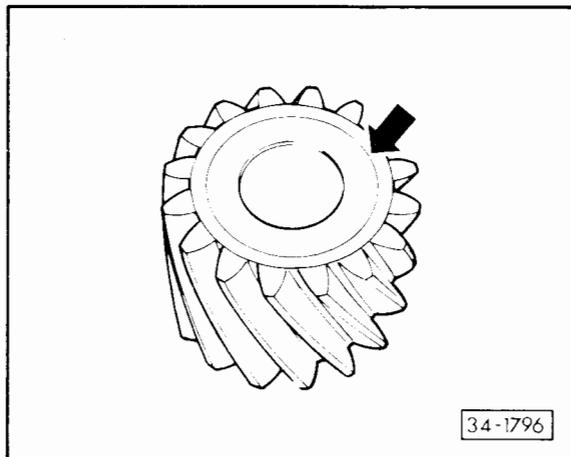
**Fig. 3 Installing reverse idler gear**
