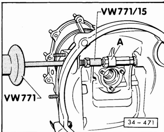
**Fig. 2 Removing bush for release shaft**
