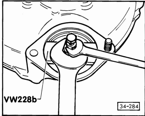
Fig. 3 Removing starter bush (gearbox installed)
