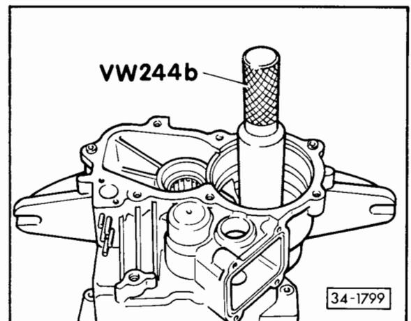
**Fig. 9 Pressing needle bearing in**
