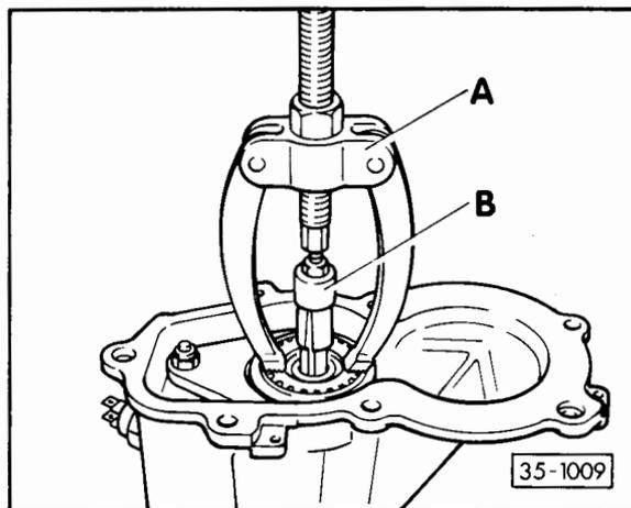
**Fig. 19 Removing needle bearing for output shaft**
