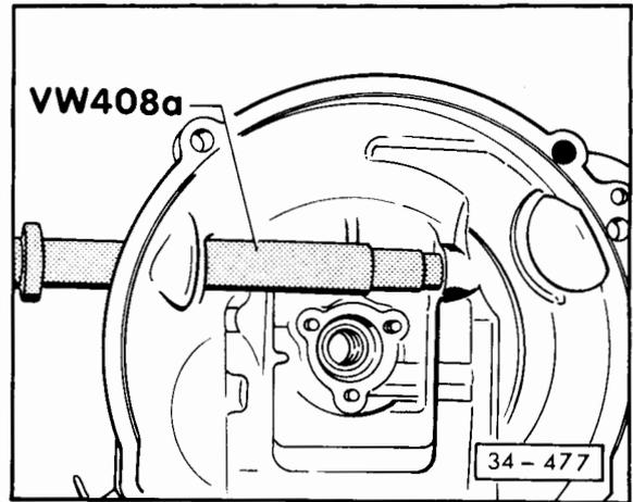
**Fig. 3 Installing bush for release shaft flush**
