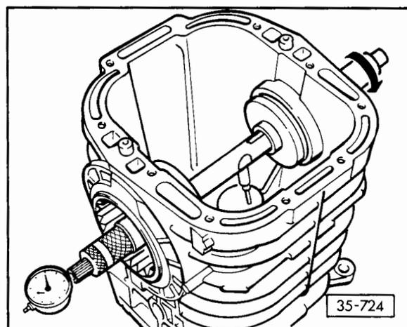
– Turn bar until measuring pin touches plate on end of pinion and needle deflects to return point.
