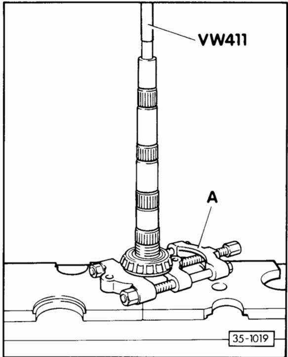
**Fig. 4 Pressing off 2nd inner race**
