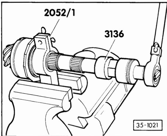
**Fig. 6 Loosening or tightening needle bearing inner race**
