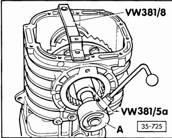
A = Torque gauge (commercially available) (0–600 Ncm)
