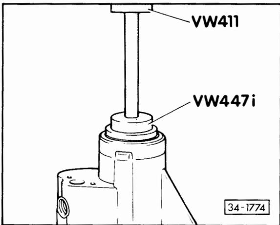
Fig. 2 Pressing deep-groove ball bearing fully home
