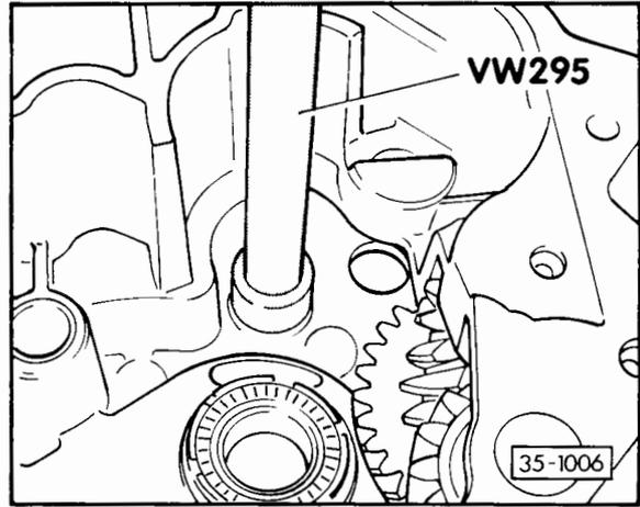
Fig. 11 Driving needle bearing into cross-country gear housing
