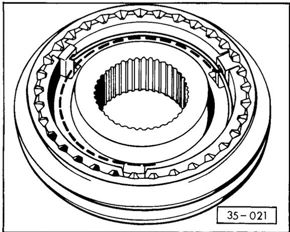
**Fig. 11 Assembling sleeve and synchronizer hub**
