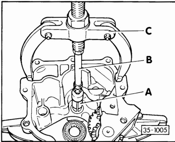
Fig. 10 Removing needle bearing from cross-country gear housing
