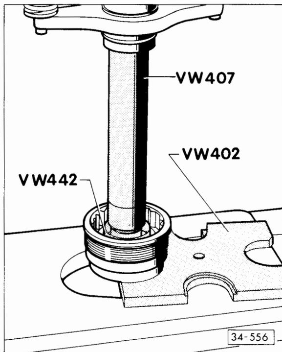
**Fig. 13** Pressing outer race/tapered roller bearing out of adjusting ring
