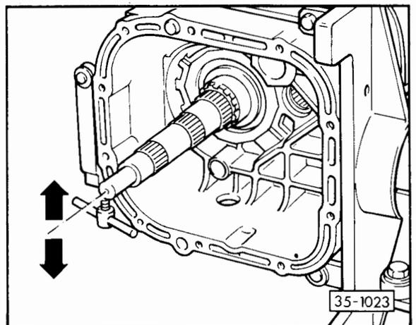
**Fig. 8 Checking rock**
