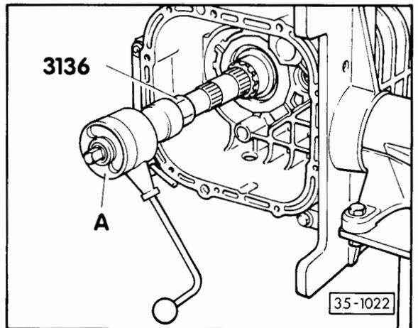
**Fig. 7 Checking turning torque of double tapered roller bearing**
