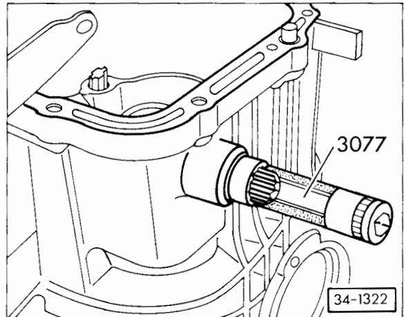
Fig. 4 Knocking in oil seal for gearshift shaft
