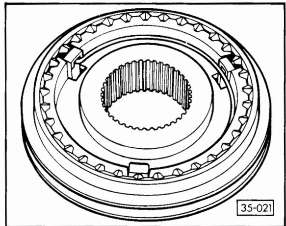
**Fig. 4** Assembling sleeve and synchronizer hub
