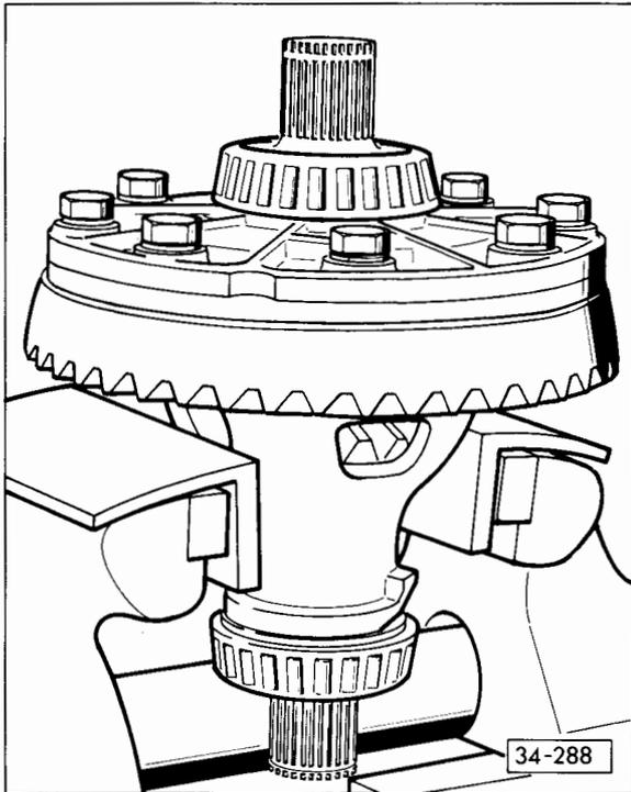
**Fig. 1 Clamping differential in vice**
