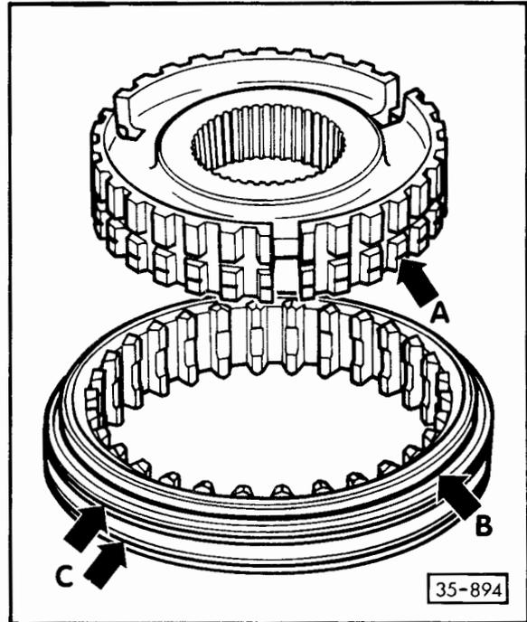
**Fig. 3** Assembling sleeve and synchronizer hub for 3rd and 4th gears
