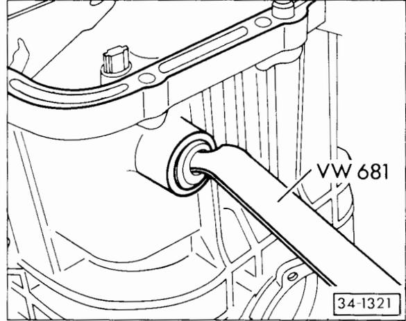
Fig. 3 Pulling out oil seal for gearshift shaft
