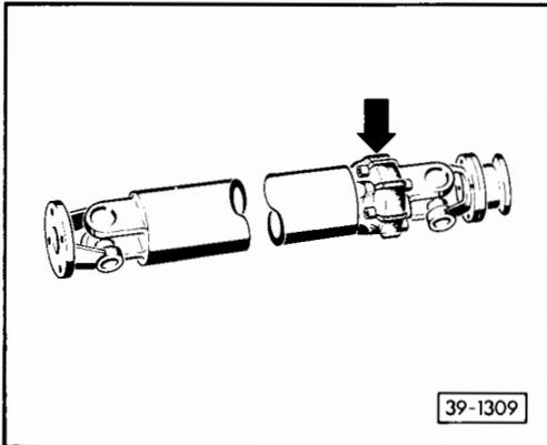
◀ The propshaft of vehicles with turbo-diesel or fuel-injection engines is fitted with a sound-proofing rubber element (arrow).
