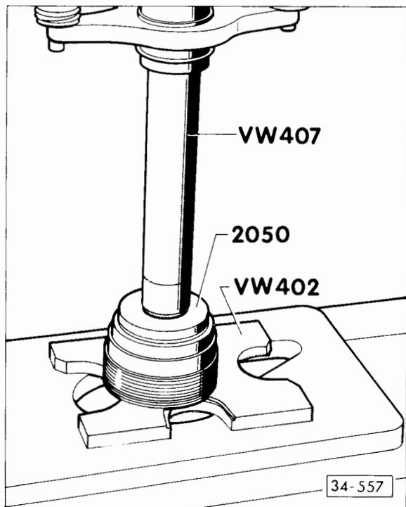
**Fig. 14** Pressing outer race/tapered roller bearing into adjusting ring
