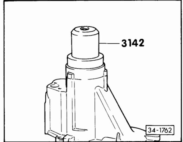
**Fig. 7 Pressing radial seal fully home**
