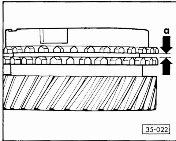
**Fig. 2** Checking synchronizer rings
