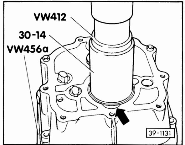
**Fig. 7 Pressing deep-groove ball bearing fully home into bearing carrier**
