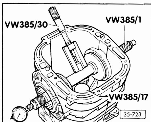
– Set universal gauge VW 385/30 to **Ro = 63.00 mm** and place it on the bar. Zero dial gauge (3 mm) with 1 mm preload.
