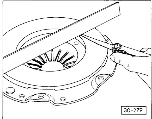
**Fig. 4 Checking the contact surface for cracks, signs of burning and distortion**
