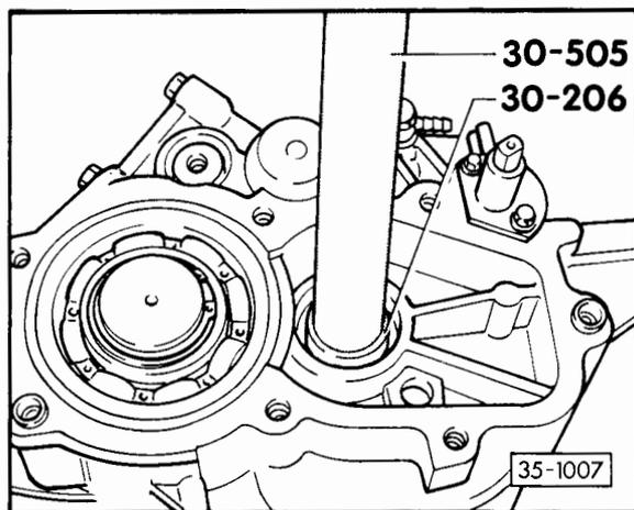
**Fig. 17 Pressing bearing out of cross-country gear housing**
