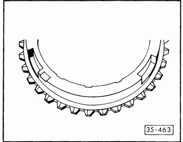
**3rd gear:** Special brass ring, sprayed with molybdenum. Full outer tooting.
