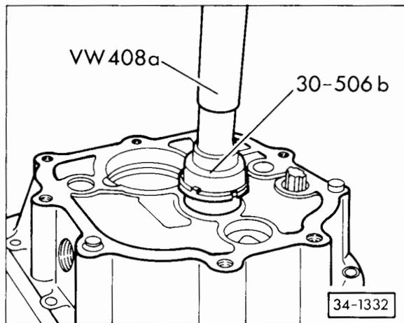
**Fig. 16 Pressing outer race/needle bearing into bearing carrier**
