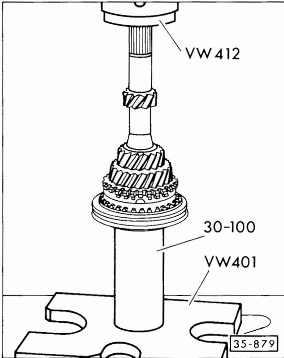
**Fig. 5 Pressing on sleeve with synchronizer hub**
