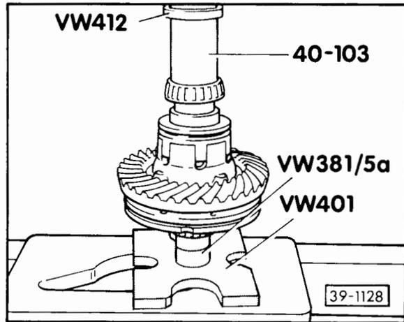
Fig. 11 Heat inner race of tapered roller bearing to about 100° C, install and press home
