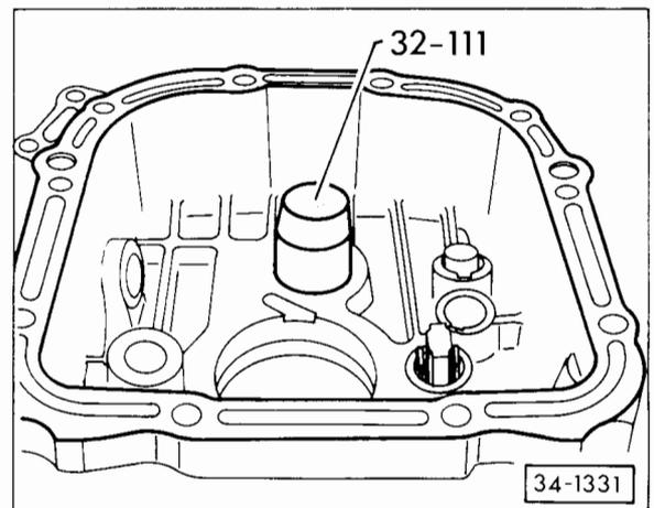
**Fig. 15 Driving outer race/needle bearing out of the bearing carrier**
