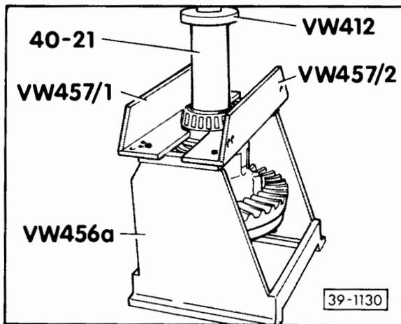
**Fig. 5 Pressing inner race/
