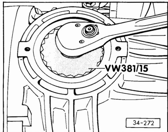
**Fig. 4 Removing adjusting rings**
