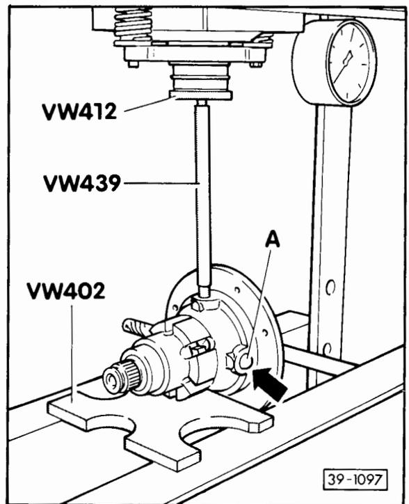
**Fig. 7 Pressing out differential pinion shafts**
