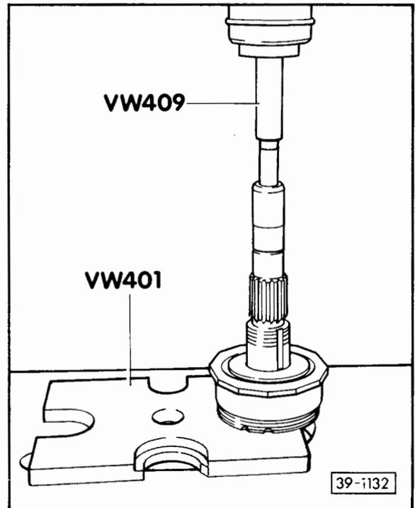
**Fig. 4 Pressing off double tapered roller bearing**
