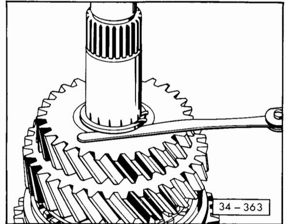
**Fig. 14 Adjusting 3rd gear wheel axial play**
