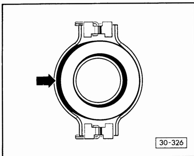
We have reason to point out that new release bearings, on which the thrust ring is not centrally positioned to the housing (arrow), can still be installed without giving any cause for concern.
