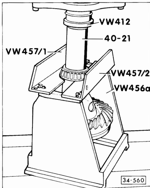
**Fig. 5 Pressing inner race/tapered roller bearing off housing**
