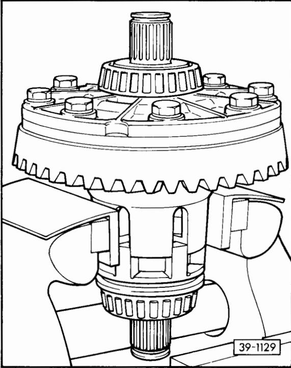
**Fig. 1 Clamping differential in vice**
