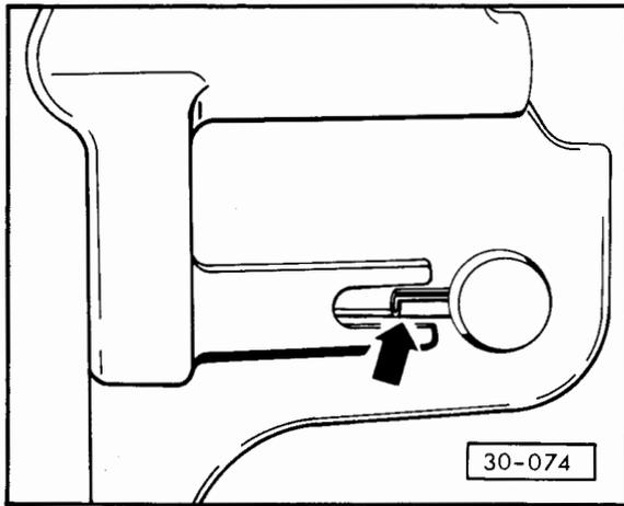
**Fig. 1 Fitting position for spring pin**
