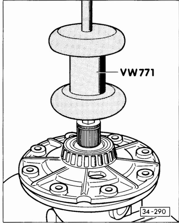
**Fig. 3 Pulling cover off differential housing**
