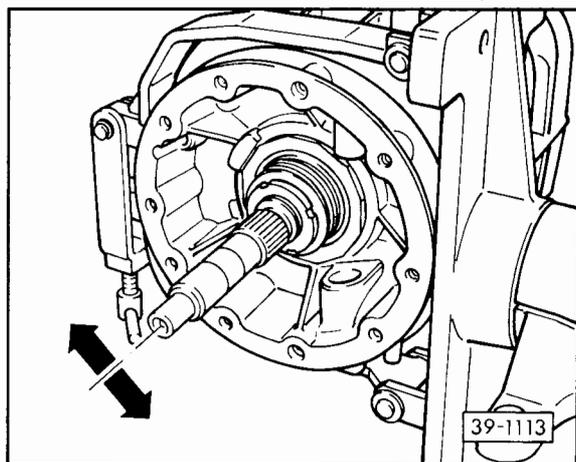
**Fig. 8 Checking rock**
