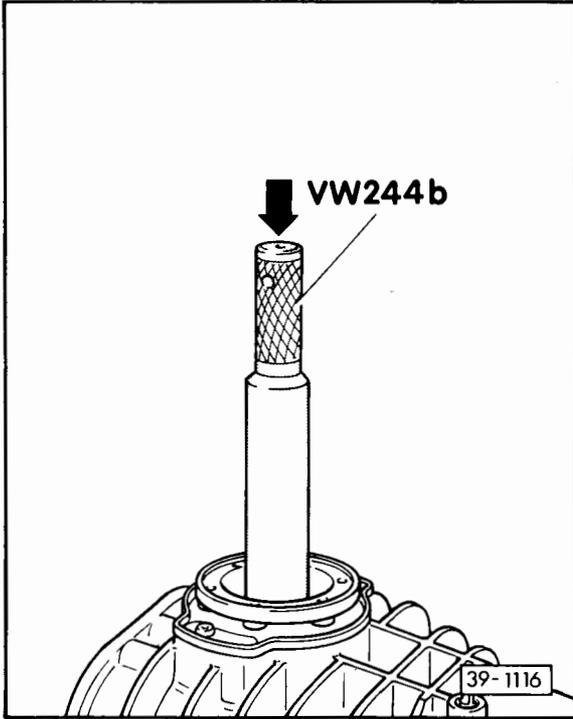
**Fig. 9 Installing circlip**
