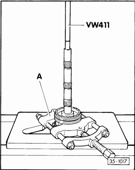
**Fig. 2 Pressing off sleeve/synchronizer hub with 1st gear wheel**
