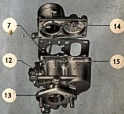
1 - Choke, 2 - Pilot jet air bleed, 3 - Float, 4 - Main jet, 5 - Volume control screw, 6 - Poppet valve, 7 - Gasket, 8 - Air correction jet, 9 - Filling tube, 10 - Emulsion tube, 11 - Idle adjusting screw, 12 - Accelerator pump, 13 - Throttle, 14 - Float needle valve, 15 - Pilot jet
