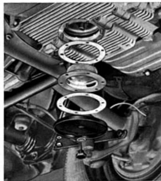
Cleaning the oil strainer.
