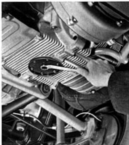
Draining the engine oil.
