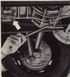
Draining the transmission oil
