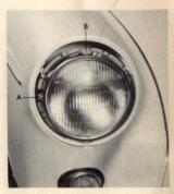
Loosen the screw in the center below the headlight and take the trim ring off.
