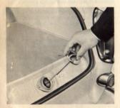
The oil level should be between the two marks on the dipstick and must never be below the lower mark. Wipe the dipstick clean before checking.
