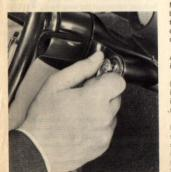
When starting the engine, the accelerator pedal must not be depressed. The amount of fuel and air required for starting is automatically supplied by the fuel injection system with which your Volkswagen is equipped.
