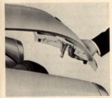
The knob which opens the front hood is on the left under the dashboard. The hood springs up slightly under spring pressure and can be opened fully when the safety hook near the lock has been pressed upward.
