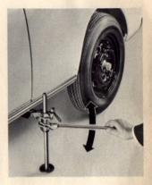
Insert jack into socket and push the jack tube down until it touches the ground.
