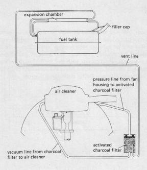
Fuel vapors pass through the filter and deposit hydrocarbons on the surface of the charcoal filter element. When the engine is running, fresh air diverted from the cooling fan of the engine cleans the filter and routes these hydrocarbons back to the engine where they are burned during normal combustion.
