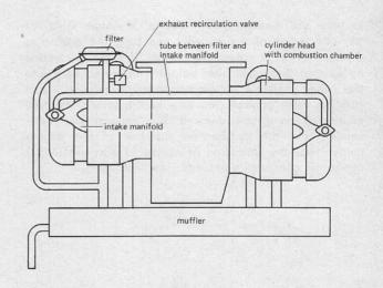
If your VW 412 is equipped with an Automatic Transmission, part of the engine exhaust is recirculated through a filter and an exhaust recirculation valve. This valve is operated by manifold vacuum. The exhaust gas enters the intake manifold to mix with the air/fuel mixture. Recirculated exhaust gas helps lower the formation of harmful oxides of nitrogen (NO<sub>X</sub>) during combustion.
