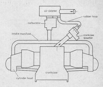
The Crankcase Ventilation System for the VW Station Wagon, Campmobile or Kombi is shown in the illustration.
