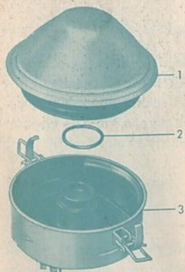
1-Filter element, 2-Gasket, 3-Oil reservoir
